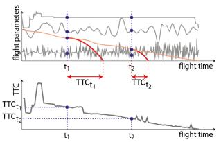
Fig. 2. Creating a time-to-crash graph (bottom) by calculating the new altitude profile (red) for the case that the flight would be resumed without any control inputs.
