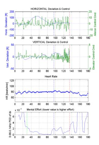
Fig. 6. Analysis of heart rate and HRV for a flight of the retired professional pilot.
