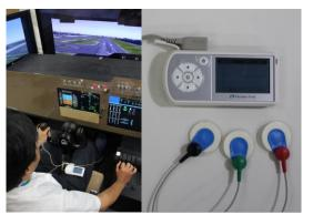
Fig. 3. The portable ECG recorder and electrode placement used when operating our fixed base flight simulator.
