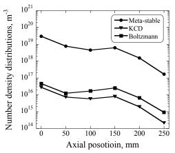
FIGURE 5. Estimated total number density distributions of xenon atom, r=30 mm.
