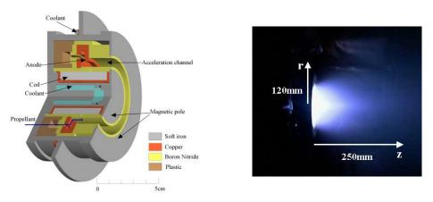
FIGURE 3. Cross sectional view of UT magnetic layer type Hall thruster (left) and its plume photo (right).
