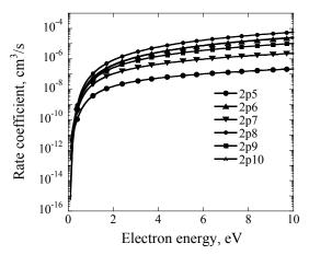
FIGURE 2. Excitation rate coefficient for electron collisions with meta-stable xenon atom.
