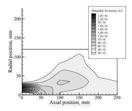
FIGURE 1. Number density distribution of meta-stable xenon (1s5) by laser absorption spectroscopy.
