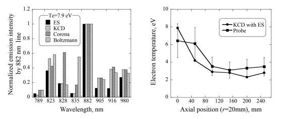
FIGURE 4. Models evaluation; relative line intensity normalized by 881.9 nm line by the experiment, KCD, corona and Boltzmann models (left) and electron temperature distributions by KCD model and single probe measurement (right).
