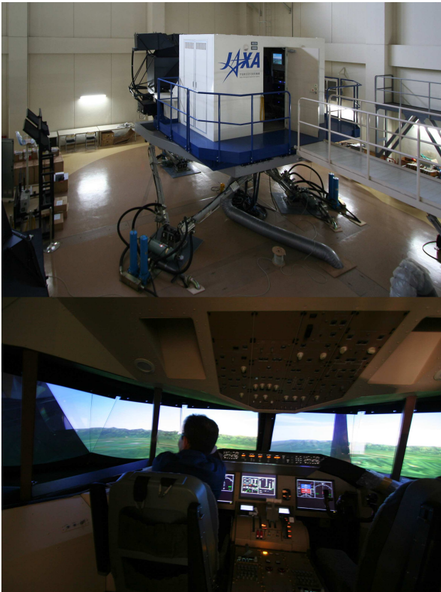
Fig. 3 The JAXA owned flight simulator used with the Dornier Do228-202 propeller airplane model and scene with rich texture.
