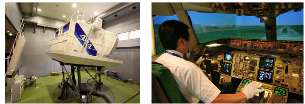
Fig. 2 Outside and inside of ANA’s Boeing 767-300 simulator
