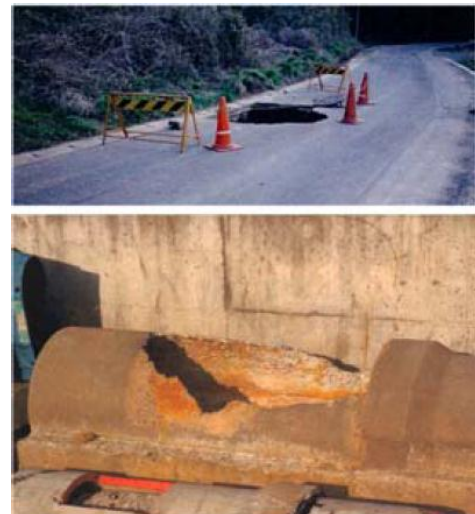
Figure 2.11: Cave-in caused by corrosion of steel pipe (Kuwano, R 2011)
