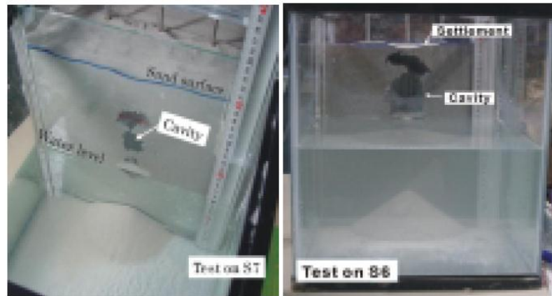
Figure 2. 27: Wall defect has caused cavity in granular backfill (Sekiguchi et al. 2003)
