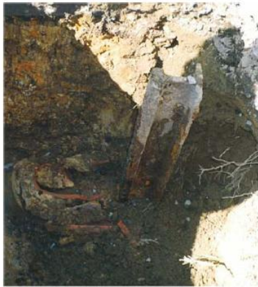
Figure 2. 13: A sewer pipe destroyed by a pile constructed for a building (Kuwano, R 2011)
