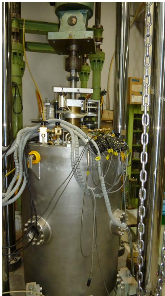
Figure 2-2: Photo of Large-scale True Triaxial Apparatus employed in this study
