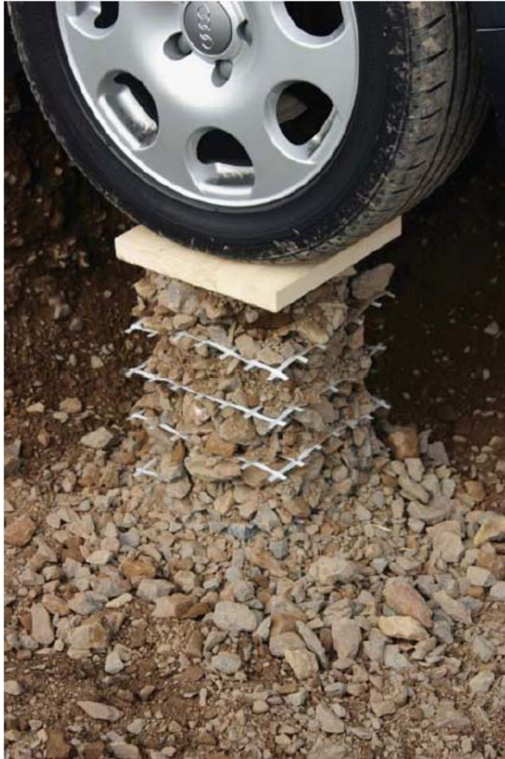
Figure 1-2: Demonstration of the interlock effect with a car standing on a laid and welded geogrid reinforced gravel column (K. von Maubeuge and C. Lesny, Mexico 2008)
