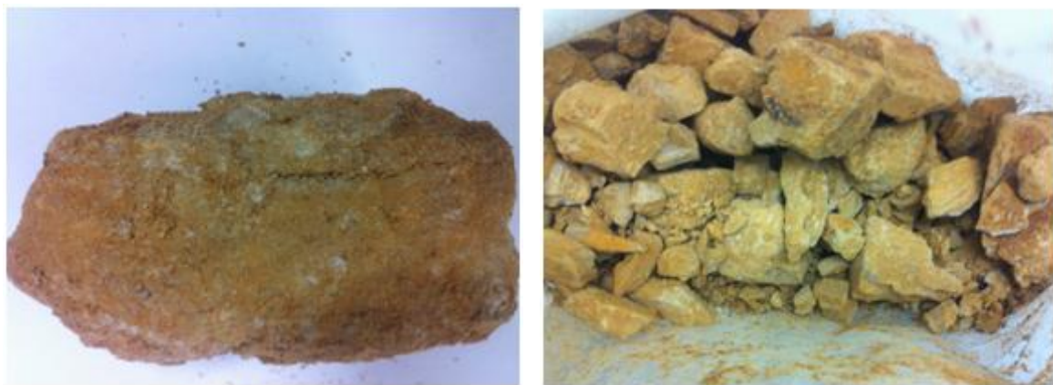
Fig. 5.1 Hattian Bala mudstone piece a) before slaking test b) after slaking test with minor cracks
