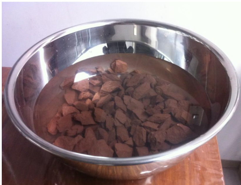
Fig. 4.17 Wetting of the Mudstone specimen in water during a slaking ratio test (Hattian Bala mudstone)
