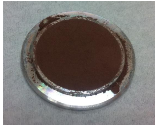
Fig. 4.20 Sample preparation for X-Ray Diffraction (Hattian Bala mudstone)
