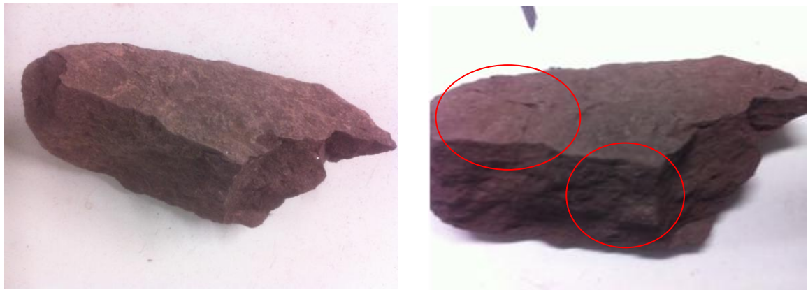
Fig. 5.1 Hattian Bala mudstone piece a) before slaking test b) after slaking test with minor cracks
