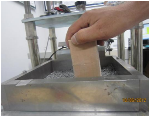
Fig. 4.33 Compaction of specimen
