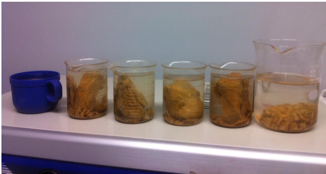
Fig. 4.16 Six set of specimens for static slaking test of Ishikawa mudstone
