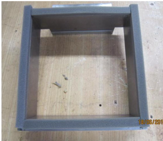
Fig. 4.29 Attached sponge to the lower periphery of the upper shear box
