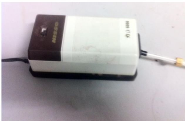
Fig. 4.39 Dry air pump to supply dry air
