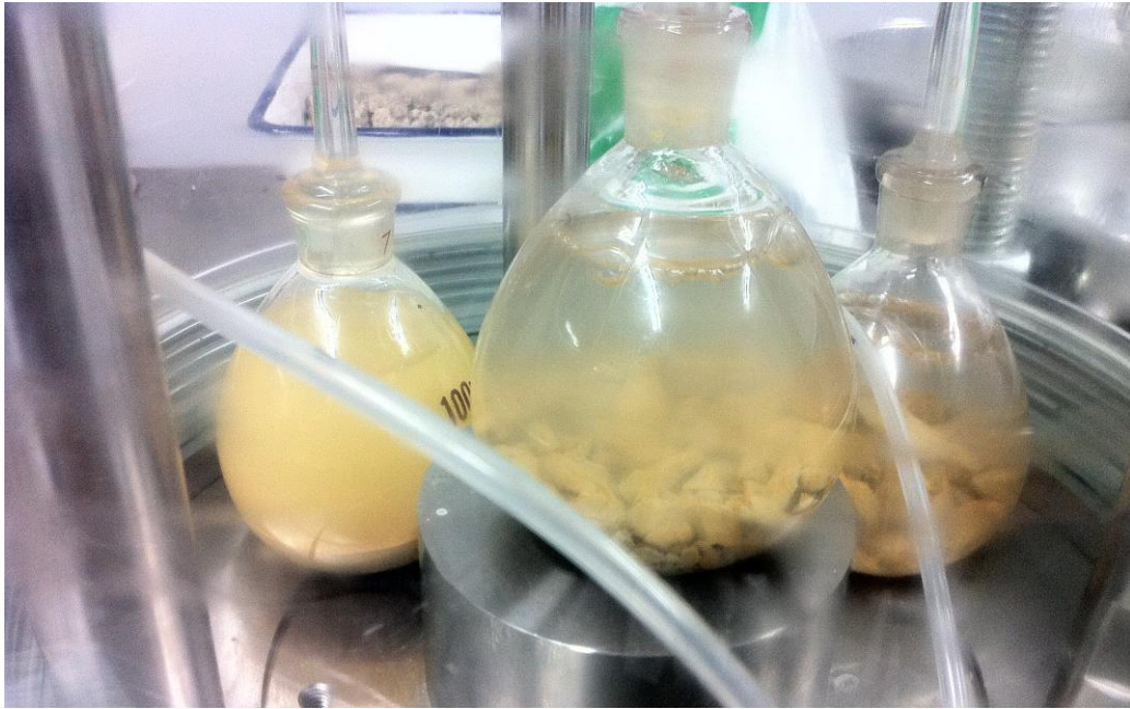
Fig 4.18 Three sets of pycnometers inside the vacuum to release air from the pores (Ishikawa mudstone)
