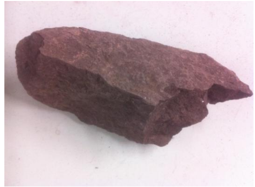
Fig. 4.15 Fresh specimen before slaking test (Hattian Bala mudstone)
