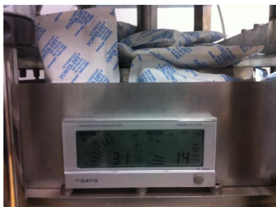
Fig. 4.41 Shear box covered by silica gel and temperature and humidity measurement
