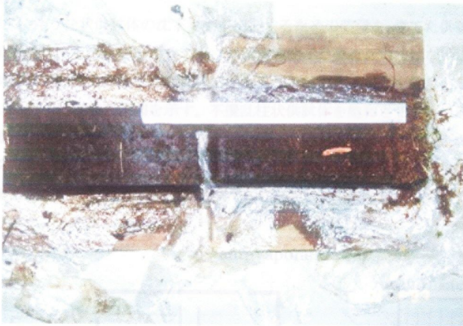
Photo 3-1 高位泥炭土柱状供試体. Parallelepiped specimen of high moor peat.
