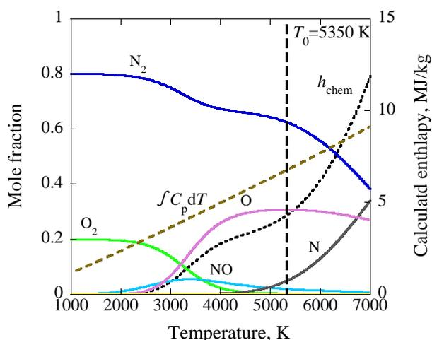
**Fig. 11** Calculated enthalpy and mole fractions by thermo-chemical equilibrium assumptions,  $p_0=23.6$  kPa.
