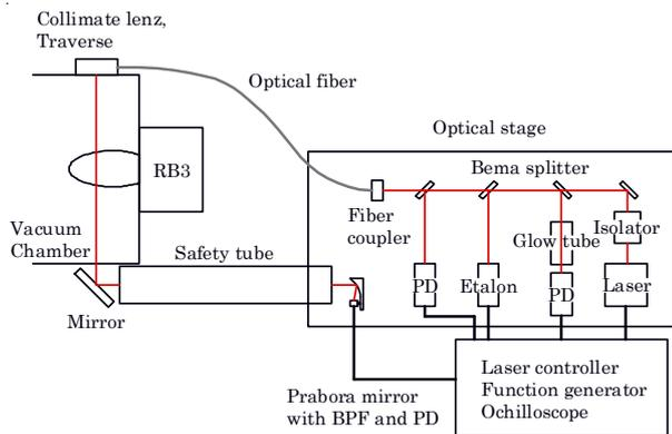
**Fig.2** LAS measurement system.
