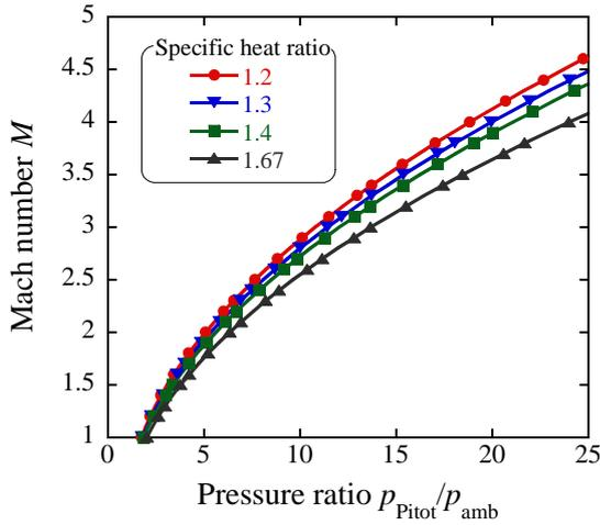
**Fig. 4** Mach number as a function of the pressure ratio for the various specific heat ratios.
