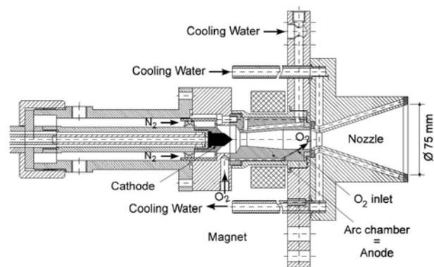
**Fig.1** A schematic of thermal arc generator RB3.
