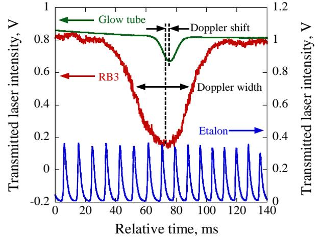
**Fig. 6** Typical transmitted laser and etalon signals.
