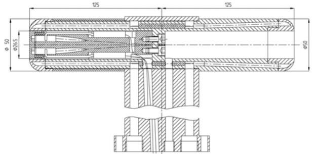
**Fig. 3** A schematic of Pitot probe.
