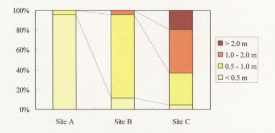
Figure 3.4-1 Slope length of levees in three study sites.
