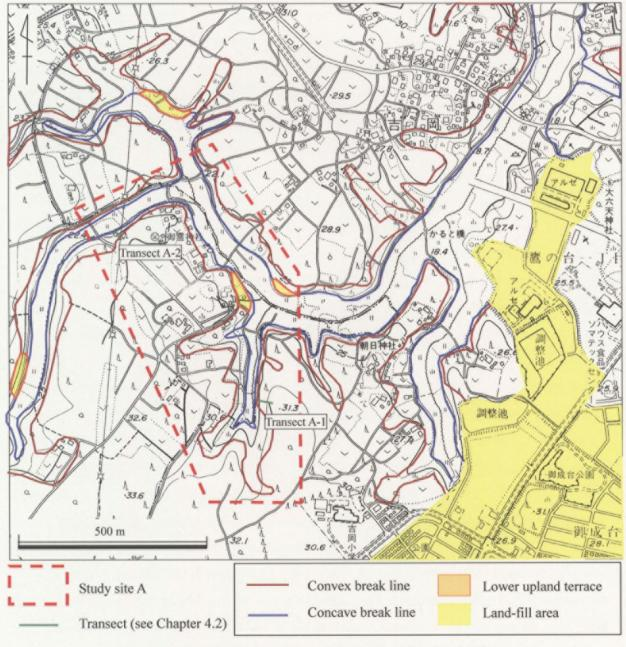
Figure 3.1-3 Detailed-scale land-form classification is Site A.
