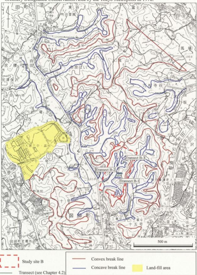
Figure 3.1-4 Detailed-scale land-form classification in Site B.
