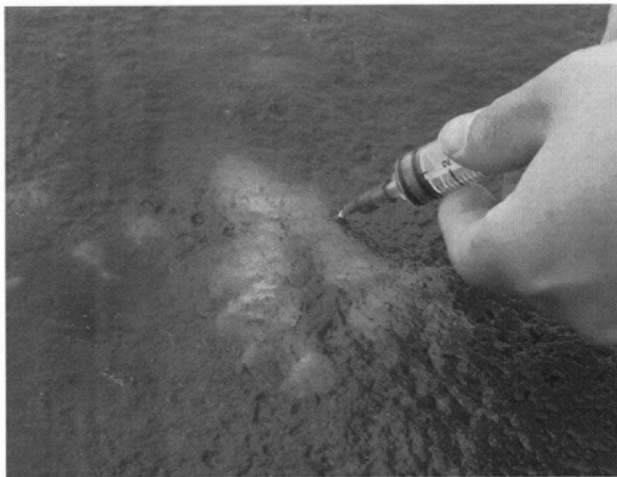
Figure5.3 Direct sampling of gaseous-phase gas (white portion) trapped between the ice and the underlying water layer conducted on April 17. The collected gas were injected in to vials and transferred to the laboratory for analysis.
