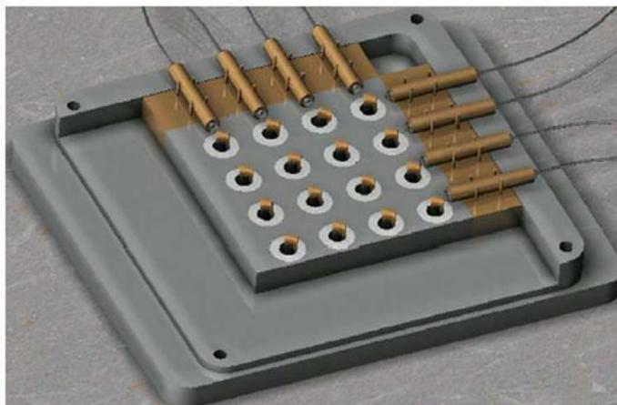
Fig 1.3 4×4 optical switch assembled with the reflection cells[6].
