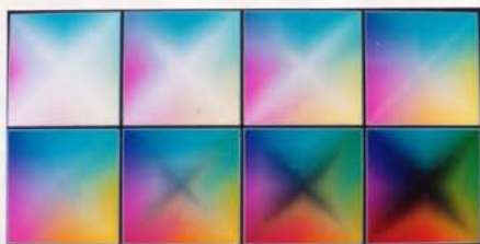
Figure 7.7. The color cube of Figure 7.6 rotated by 45^\circ about the G axis
