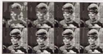
Figure 4.8. Increasing both spatial and gray scale resolution (bytes transmitted: 300, 600, 1200, 1800, 2400, 3600, 4800, 9600)
