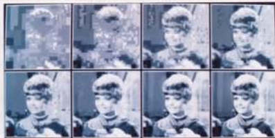
Figure 5.5. Reproduction using trace averages (bytes transmitted: 300, 600, 1200, 1800, 2400, 3600, 4800, 9600)
