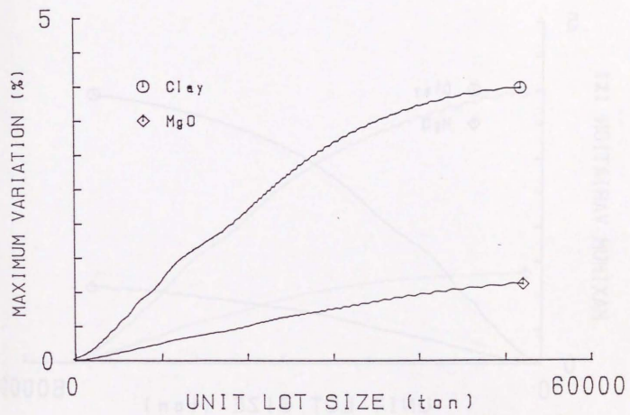
fig.5-14 The relationship between the unit lot size and the maximum quality difference. Ore blocks A,B,C and D dumped with order of A,C,D and B.
