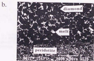
Fig. 1. (a) Three different configurations of charges used in the present experiments described in (Johnson and Kushiro, 1992; Kushiro and Hirose, 1992). Melts in equilibrium with the host peridotite can be obtained with configurations (ii) and (iii). (b) Backscattered electron image of a charge obtained at 15 kbar and 1400°C. It shows that melts are segregated and trapped between the diamond grains.
