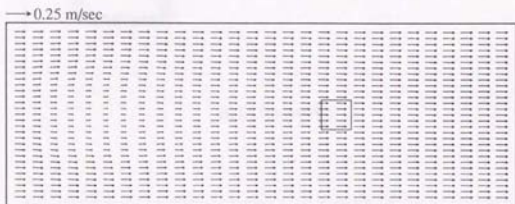
Figure 6.1.10 Computed initial water velocity distribution, Free drift of rectangle floe models
