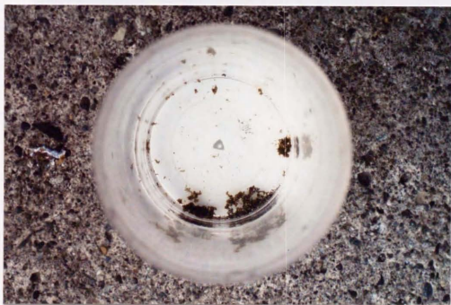
Figure 1-4. Sediment trap cylinder (a) and obtained particles at the bottom of it (b)
