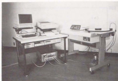
Fig. 3.2 The whole system of the "ESR dosimetry system". The remodeled ESR spectrometer is on right, and the personal computer and auxiliary equipment are on the left.
