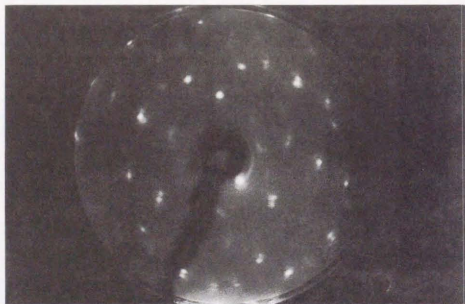
Fig. 3.14 LEED patterns of graphite / WC( 10\bar{1}0 ). E_0 = 122.8 \text{ eV} .
