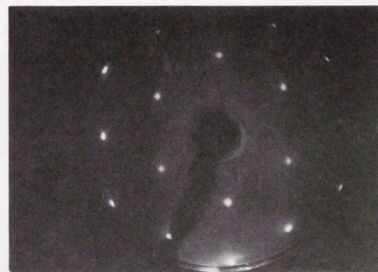
Fig. 3.2 LEED patterns of (a) clean TiC(001) and (b) TiC(111). Primary electron energies for each patterns are 204.9 eV and 229.1 eV, respectively.
