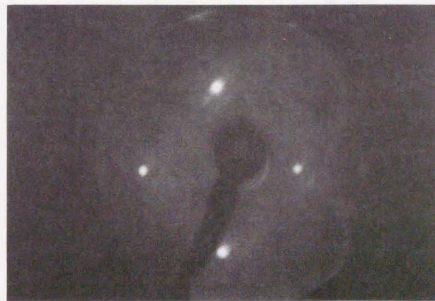
Fig. 3.15 LEED pattern of graphite / Ni(001). E_0 = 134.6 \text{ eV} .
