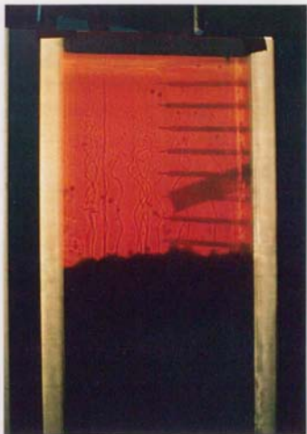
Plate.4-2. Shadow graph at 120 min in the experiment using 28 wt% floor solid. Upwelling compositional plumes from the mush front can be observed.
