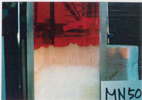
Plate.3-5. The floor experiment at 120 min. The mush above the solid front and the conduits in the mush which is called "chimneys" can be observed.
