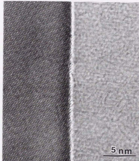
Fig.3.2 HREM image of a grain boundary in high-purity Al 2 O 3 .
