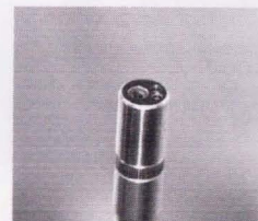
图 7.21. The head of endoscope. Larger circular hole at the left side on the head is object lens of image sensor, and two smaller ones at the right side are lens to radiate. The diameter of this endoscope head is 12mm.
