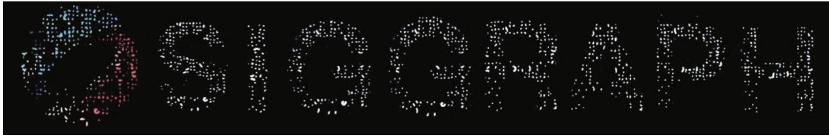
Figure 4.19: Mid-air screen with projection (showing SIGGRAPH logo, S, I, G, G, R, A, P, and H). This figure is taken separately and after that we merged into one figures. This figure is realized by floating screen filled with particles (particle is floating in dark part of this figure) and we projected image on it.
