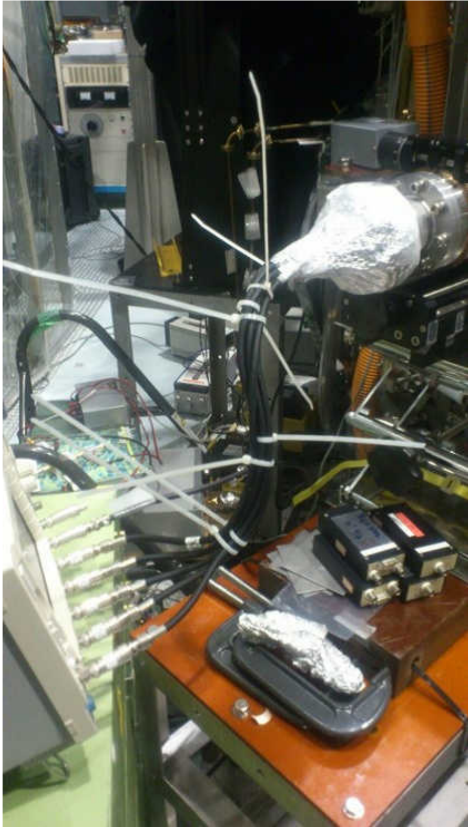
Figure 8.10: Provision for noise suppression.
