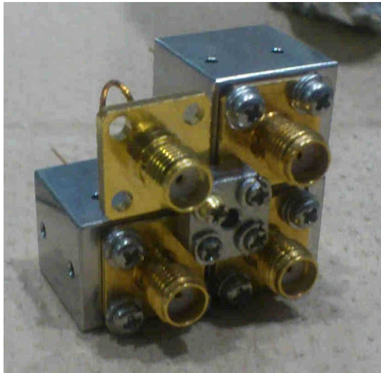
Figure 6.3: Back view of the probes held together by a SUS304 piece.
