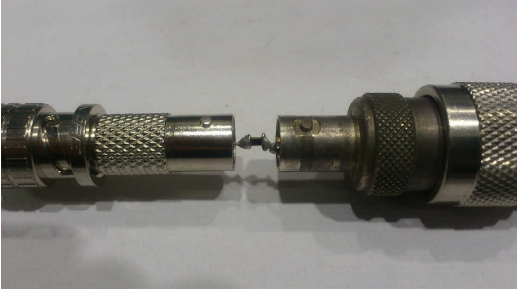
Figure 5.7: Chip resistor connection.
