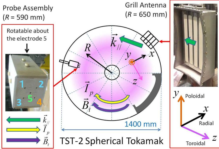
Figure 3: Cross sectional view of the experimental configuration as seen from the top.  $k_{\parallel}$ : wavenumber component parallel to the toroidal magnetic field,  $I_p$ : plasma current, and  $B_t$ : toroidal magnetic field.
