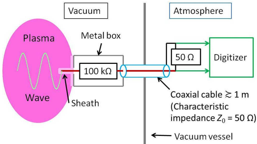
Figure 1: Proposed configuration for floating potential ( $V_f$ ) measurement at high frequencies such as 200 MHz, with a high impedance resistor between the probe electrode and the signal transmission cable.
