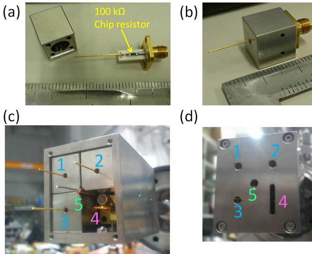
Figure 2: Photographs of the probe unit and the probe assembly. (a) Probe circuit with a high impedance chip resistor and a stainless steel (SUS304) shield box. (b) Assembled unit (high impedance Langmuir probe unit). (c) Probe assembly with the three high impedance Langmuir probes units (electrodes 1, 2, and 3), the magnetic probe (electrode 4), and the plain Langmuir probe (electrode 5). (d) Probe assembly with the stainless (SUS304) cover attached, showing the holes and the slit.
