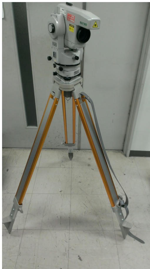
Figure 6.3: Photograph of SLT20. It was used for triangulation.
