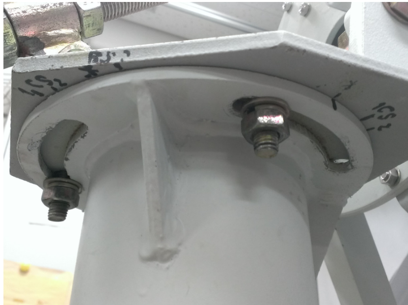
Figure 5.18: The adjustment mechanism for azimuth angle.
