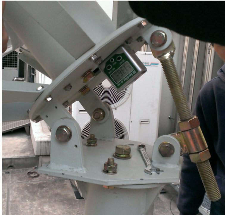
Figure 5.17: The adjustment mechanism for elevation angle.
