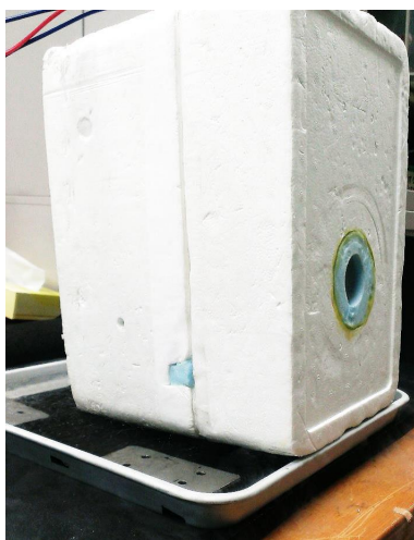
Figure 5.13: Photograph of the measurement for eccosorb at LN temperature.
