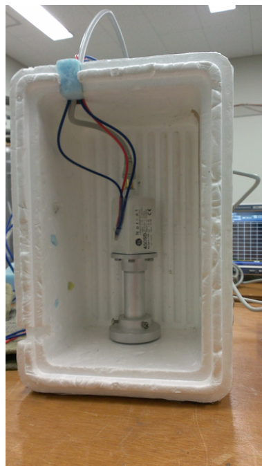
Figure 5.10: The receiver fixed in the Styrofoam box.
