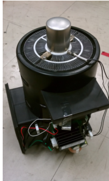
Figure 5.9: The devices for temperature control. The left one is cement resistor for heating and the right one is Stirling refrigerator for cooling.
