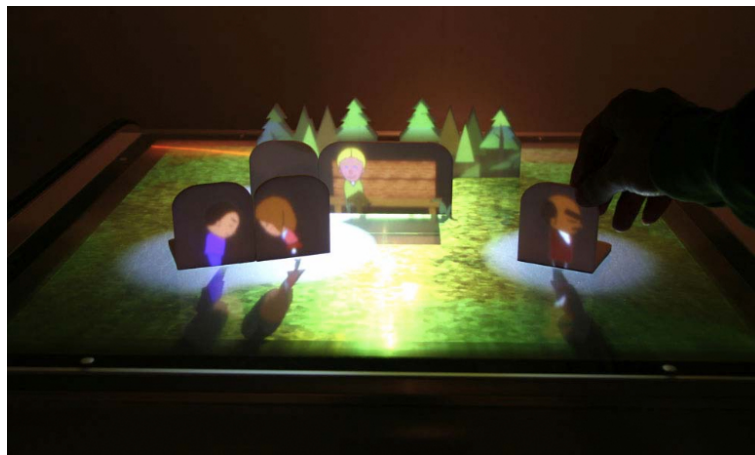
Figure 2.23: Tablescape Plus by Kakehi et al. [49]. Characters are projected to tiny upright screens on the table. Horizontal images are displayed from the tabletop surface.
