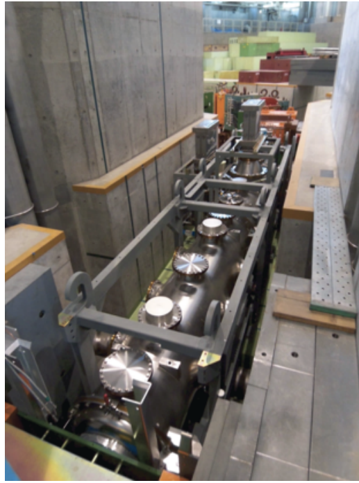
Figure 2.12.: Photograph of the first stage electrostatic separator of the K1.8 beam line viewed from upstream [62].
