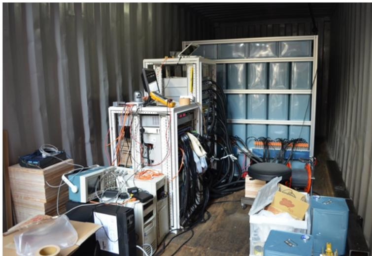
Figure 3.2: PANDA64 and water shield loaded on a 12 feet container
