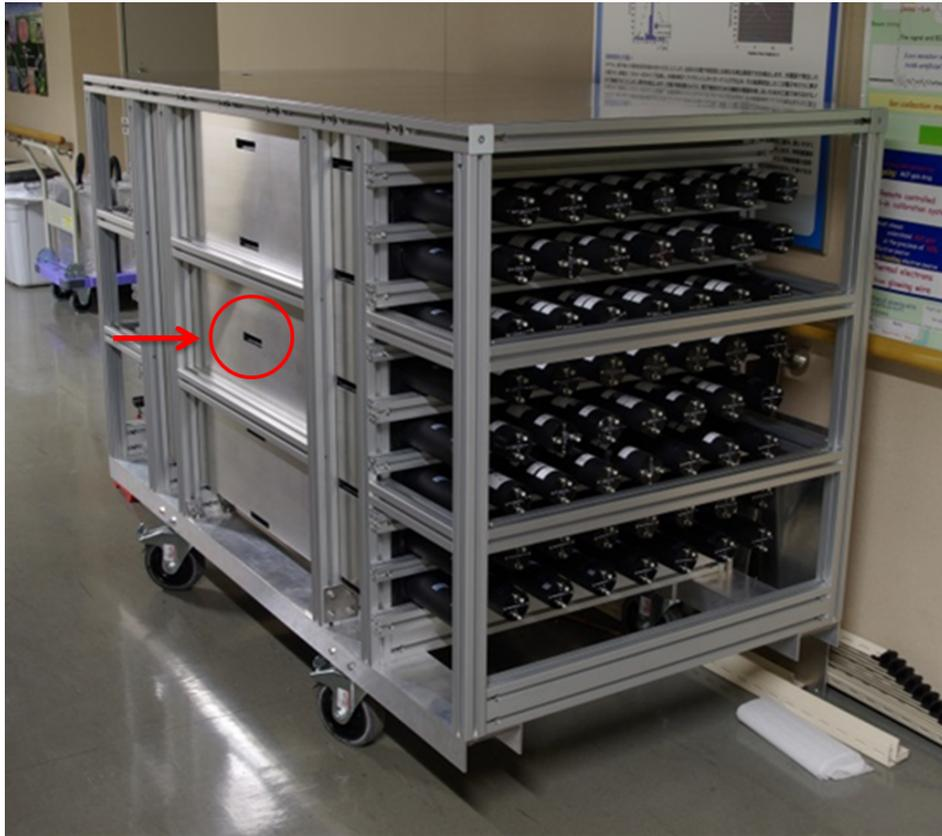
Figure 3.1: The third prototype PANDA64 consists of 64 modules. Red circle shows a slit for calibration sources.
