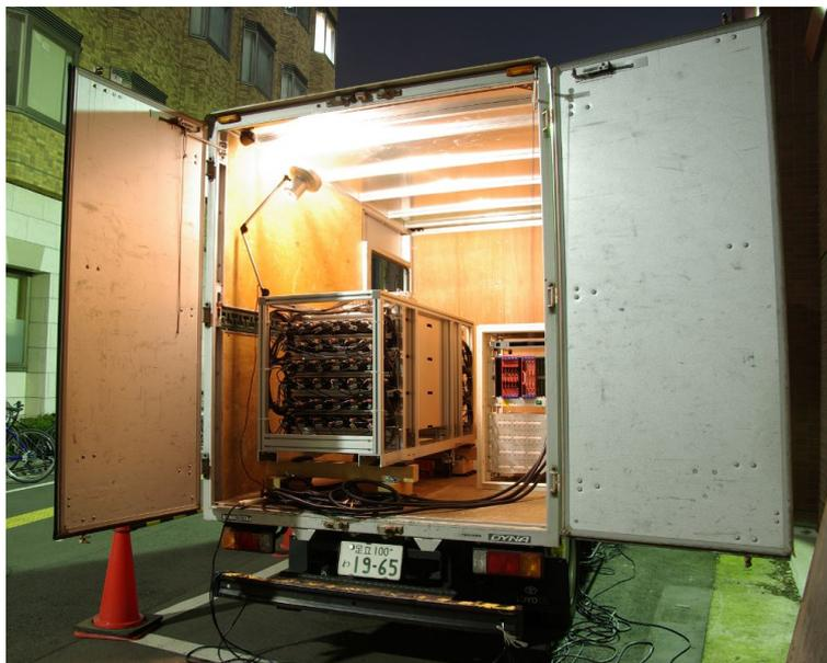
Figure 2.8: PANDA36 loaded on a 2 ton van before transportation to Ohi Power Station
