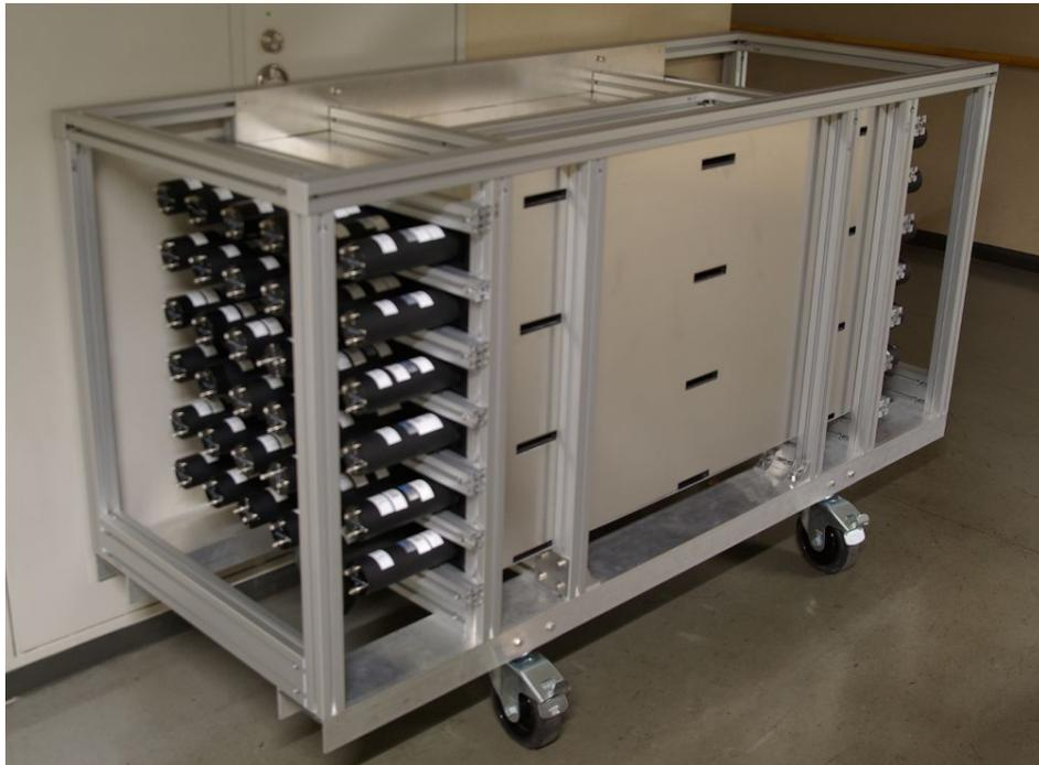
Figure 2.7: The second prototype PANDA36 consisted of 36 modules.
