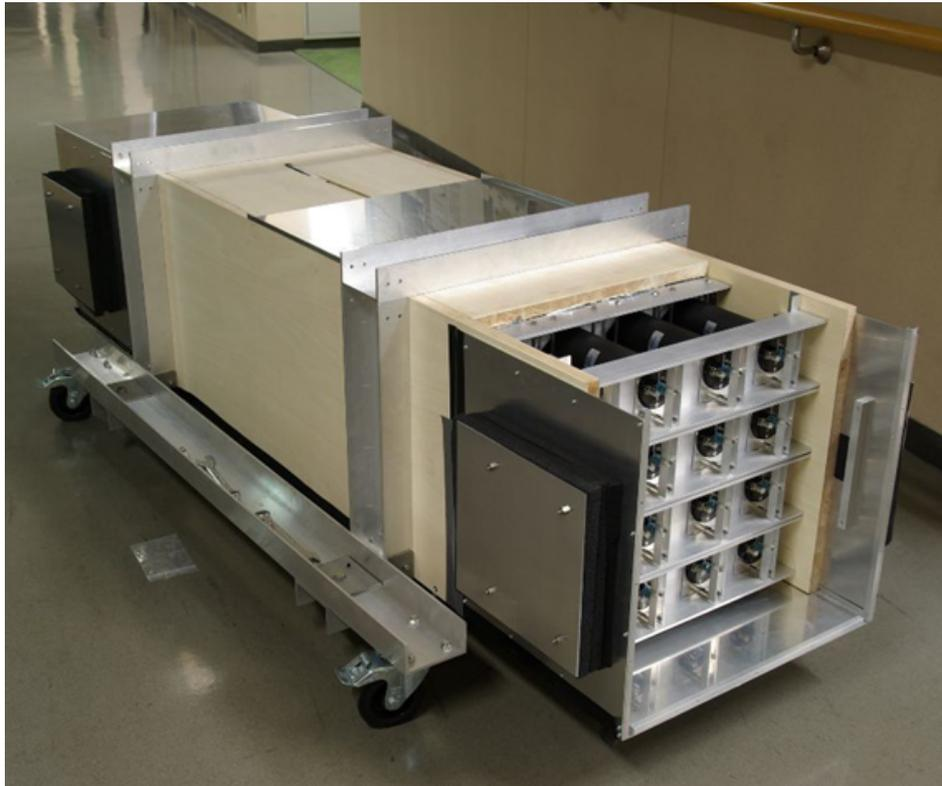
Figure 2.4: The first prototype (LesserPANDA) : LesserPANDA consisted of 16 modules.
