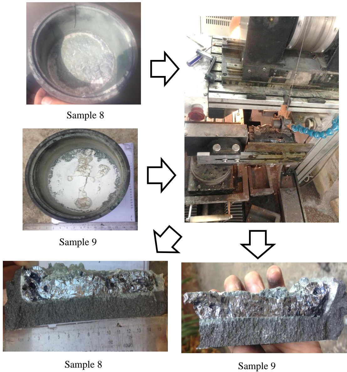
Figure 5.10 Cut of Silicon using wire cutting machine
