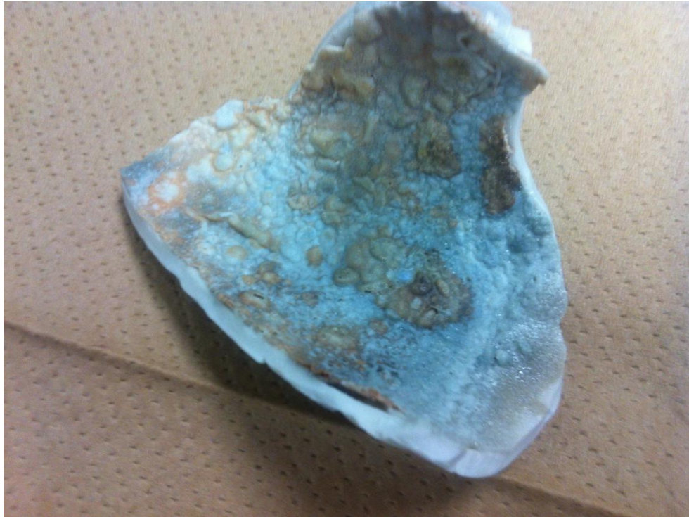
Figure 2.9. Precipitant attached on the alumina ceramic tube
