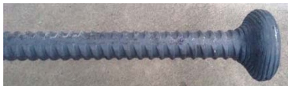
Fig. 8.1 Mechanical anchorage
