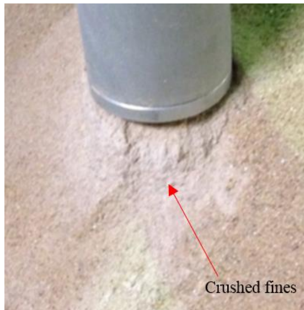
Figure 6.25 Notable sand crushing observed below the pile tip after pile penetration
