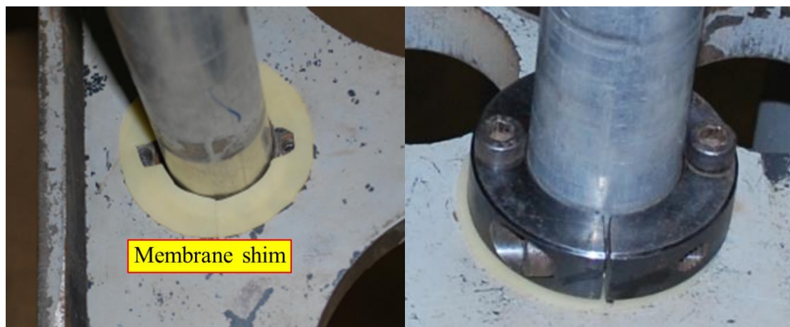
Figure 4.14 Membrane shim placed between footing and fastening bolt
