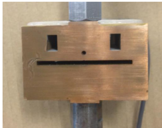
Figure 3.4 Axial load cell employed in small pile testing system
