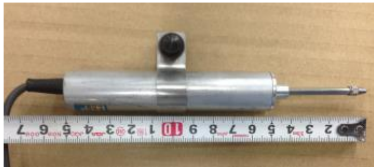
Figure 3.6 EDT used in small pile testing system
