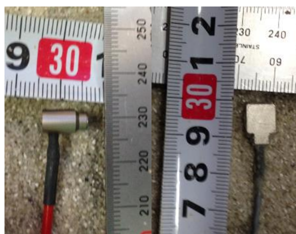
Figure 4.9 Sensor set-up for AE source location
