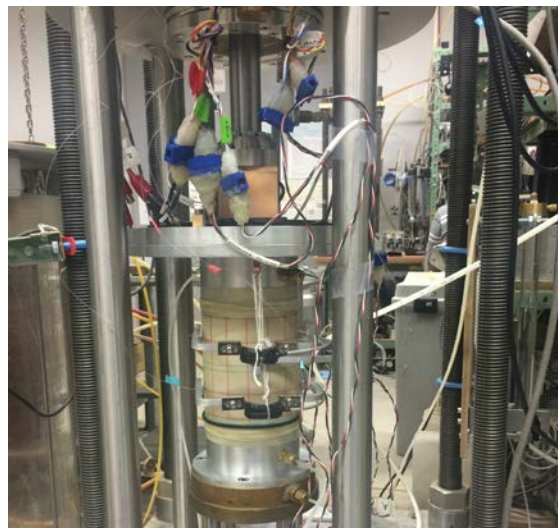
Fig. 3.34 Tow-component load cell and the specimen
