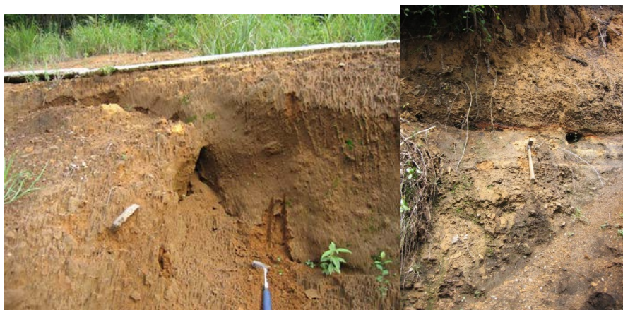
Fig. 2.2 Piping holes observation after the heavy rain in Kagoshima (1993)
