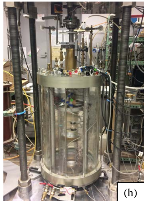
Fig. 3.52 Preparation of specimen in hollow cylindrical torsional shear apparatus
