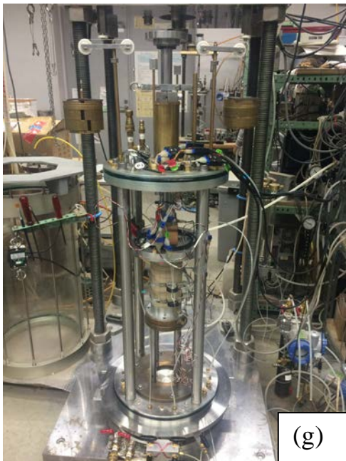
Fig. 3.52 Preparation of specimen in hollow cylindrical torsional shear apparatus
