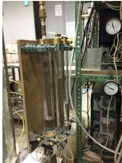
Fig. 3.35 Low Capacity Differential Pressure Transducer
