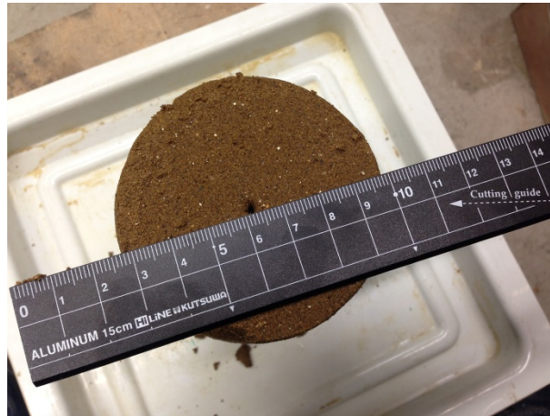
Fig. 5.46 Piping propagation in Edosaki sand
