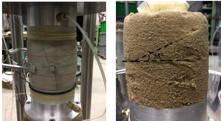
Fig. 6.32 Shear band in specimen with horizontal pipe
