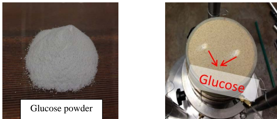
Fig. 3.5 Vertical glucose pipe in triaxial apparatus
