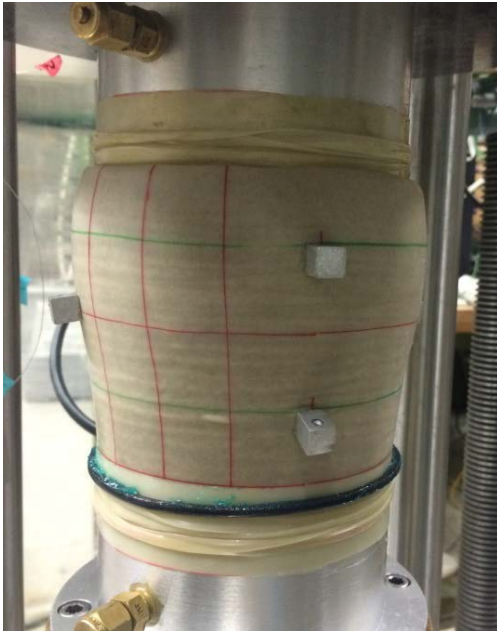
Fig. B-1 Shear band in No-pipe-specimen for (a) \alpha = 0^\circ and (b) \alpha = 45^\circ
