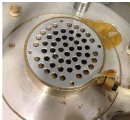
Fig. 2.6 Suffusion simulation through modified pedestal in triaxial apparatus (Sato. M, 2014)
