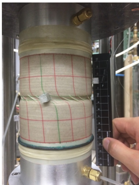
Fig. B-3 Shear band in Horizontal-pipe-specimen for (a) \alpha = 0^\circ , (b) \alpha = 45^\circ , (c) \alpha = 60^\circ and (d) \alpha = 90^\circ
