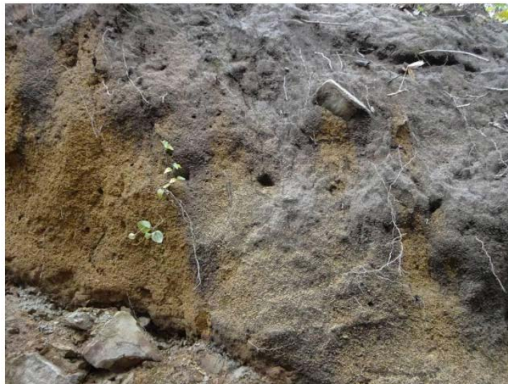
Fig. 1.4 Piping holes in the topsoil layer
