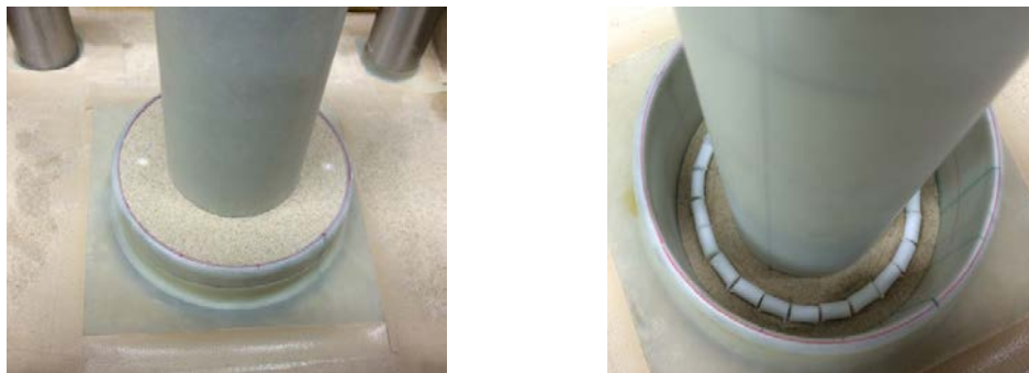
Fig. 3.6 Vertical & horizontal glucose pipe in torsional shear apparatus
