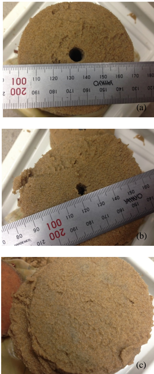
Fig. 5.45 Piping propagation in Toyoura sand (a: top; b: 12mm from the top; c: bottom)
