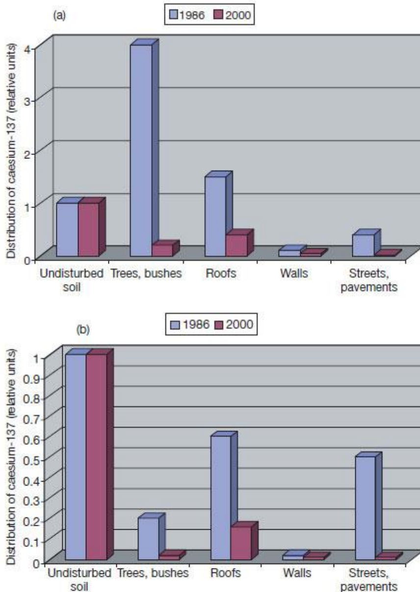
FIG. 3.10. Typical distribution of ^{137}\text{Cs} on different surfaces within settlements in 1986 and 14 years after deposition of the Chernobyl fallout. (a) Dry deposition; (b) wet deposition [3.23].
