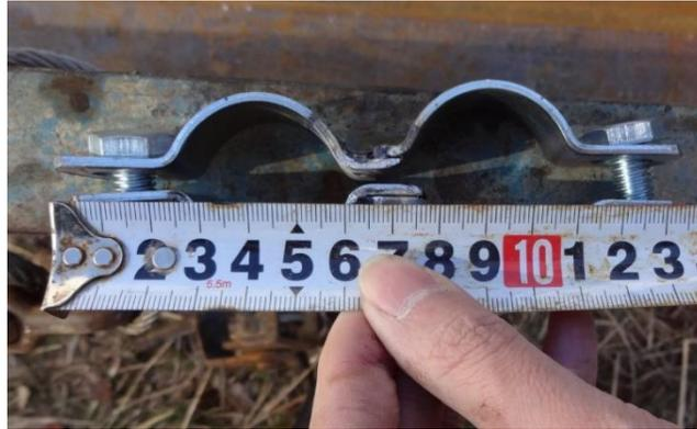
**Fig. 3.3** Spacer used to maintain shank space of U-tube (units of ruler: cm).
