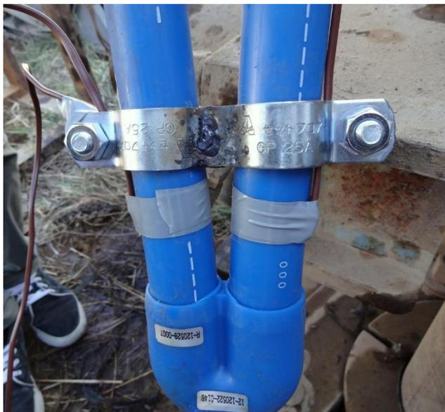
**Fig. 3.5** T-type thermocouples installed on surface of U-tube.
