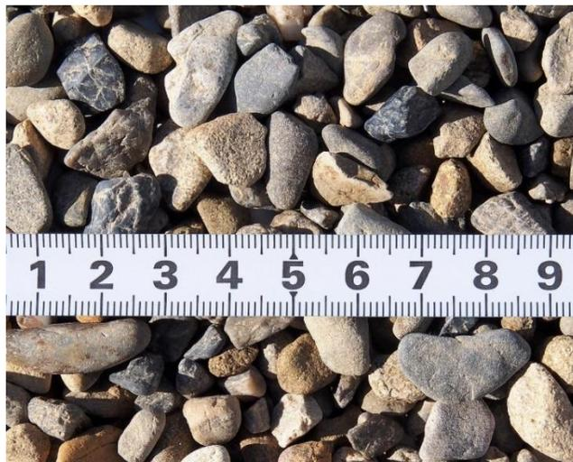
**Fig. 3.4** Grain size of the gravel used in backfilled BHE (units of ruler: cm).
