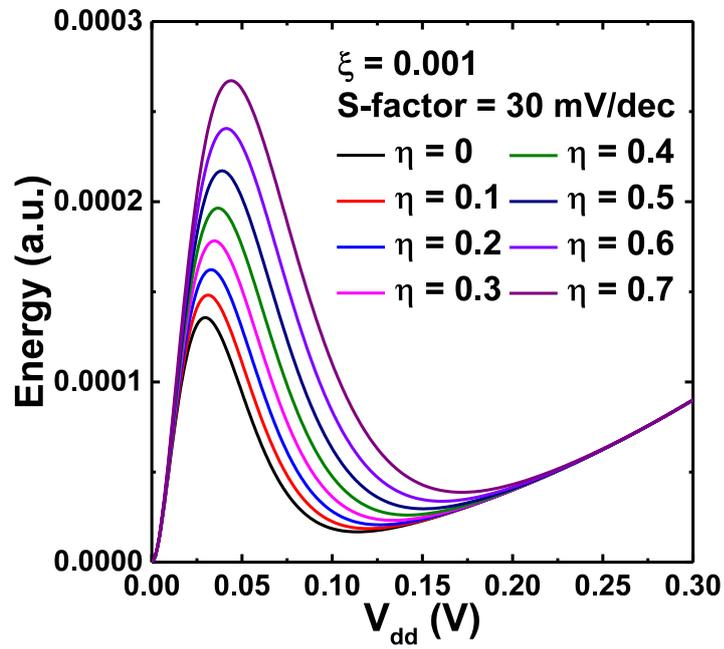
Figure 3.5 Calculated  $V_{dd}$  dependence of energy at s-factor =30 mV/dec with various  $\eta$  factors. The optimal points of  $V_{dd}$  and energy consumption become larger with  $\eta$  factor increase.
