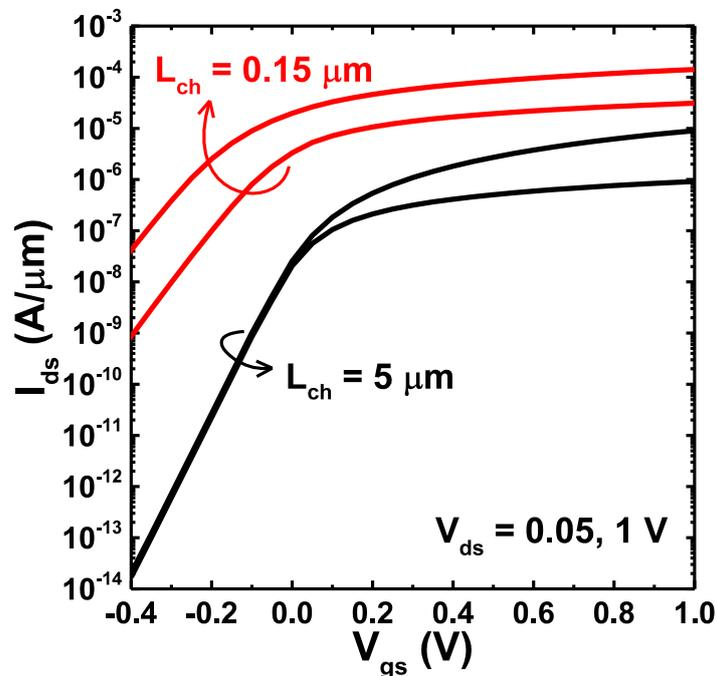
Figure 4.11 Simulated transfer curves of  $V_{th}$  self-adjusting MOSFETs with  $L_{ch} = 5$  and  $0.15 \mu\text{m}$ .
