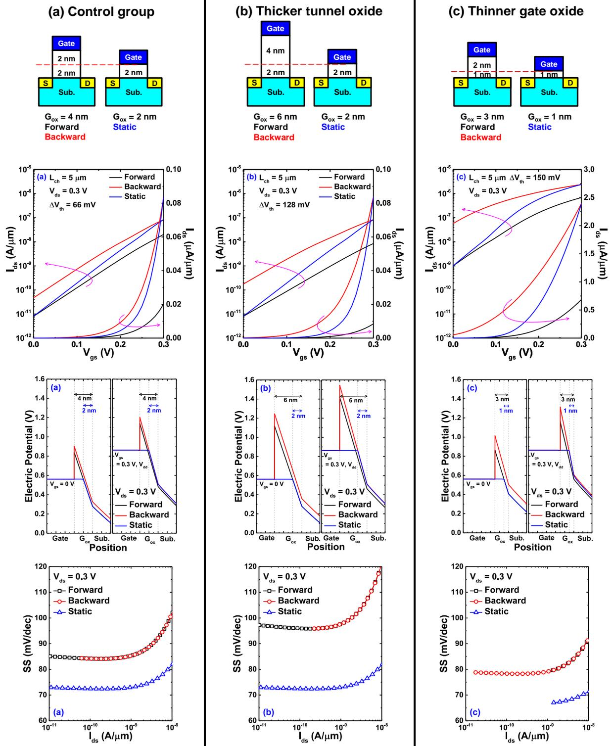
Figure 4.5 Simplified modeling structure and its transfer curves, electric potential and s-factor of  $V_{th}$  self-adjusting MOSFET at  $V_{dd} = 0.3$  V with (a) control group, (b) thicker tunnel oxide and (c) thinner gate oxide.
