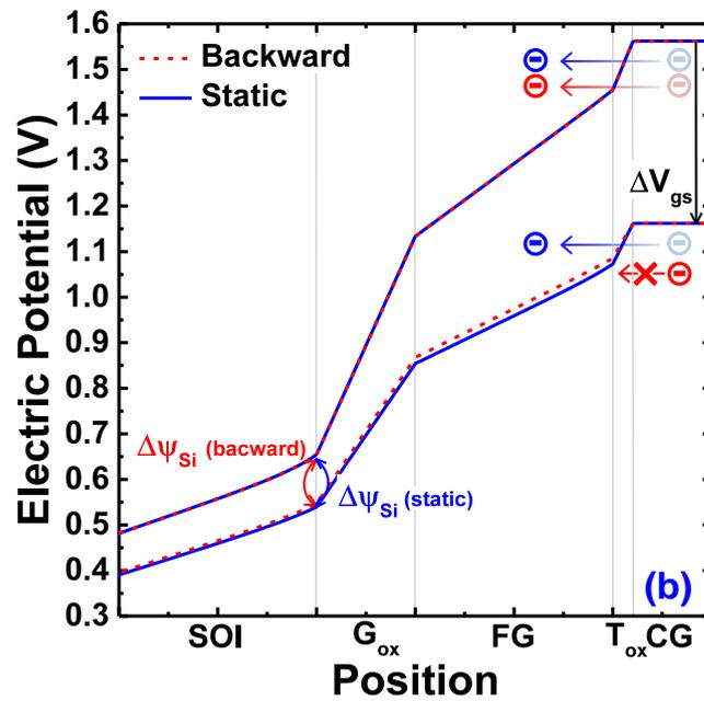
Figure 4.3 Electric potential between dynamic ((a) forward, (b) backward) and static characteristics in case of nMOSFET. The tunneling of electrons is under the control by time-lag.
