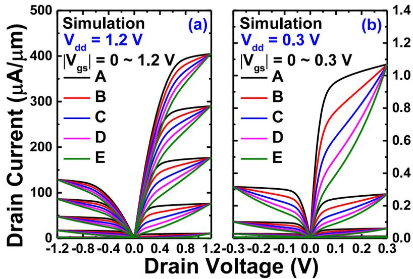
Figure 2.8 Simulated output curves with various DIBL of (a) above threshold region ( $V_{dd} = 1.2$  V) and (b) subthreshold region ( $V_{dd} = 0.3$  V). Current at  $|V_{ds}|/2$  is degraded by DIBL increase, particularly at  $V_{dd} = 0.3$  V.
