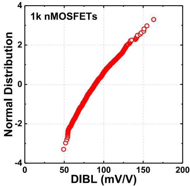
Figure 2.1 Normal distribution of DIBL from 1k bulk nMOSFETs fabricated by the 65 nm technology. The DIBL distribution is caused by unbalanced impurities location in the channel.
