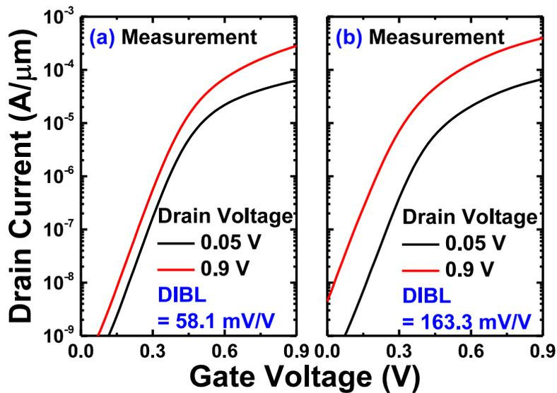
Figure 2.2 Transfer curves of measured bulk nMOSFETs with (a) small (58.1 mV/V) and (b) large DIBL (163.3 mV/V).
