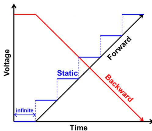
Figure 4.2 Sweep time and voltage sequence of dynamic (forward, backward) and static characteristics. There is time-lag between dynamic and static characteristics except initial point.
