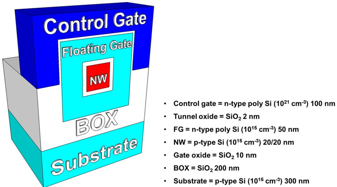
Figure 4.13 Three-dimensional schematic structure of proposed tri-gate nanowire MOSFET with floating gate to suppress short channel in  $V_{th}$  self-adjusting MOSFETs.
