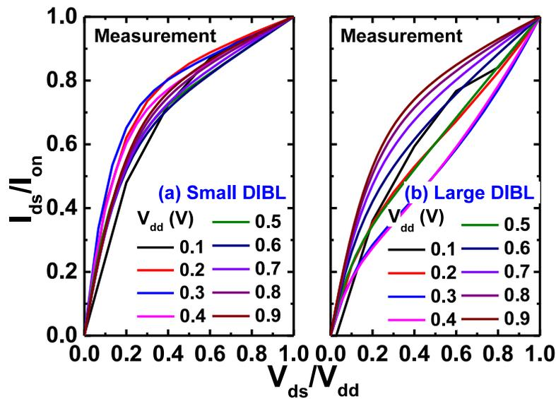
Figure 2.4 Normalized output curves of measured bulk nMOSFETs with various  $V_{dd}$ . (a) shows small DIBL and (b) shows large DIBL. Large DIBL device shows more variation in performance.
