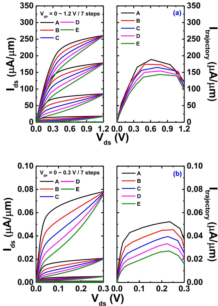
Figure 2.11. Simulated output curves and trajectory current with various DIBL at (a)  $V_{dd} = 1.2$  V and (b) 0.3 V. The degradation of trajectory current by DIBL at  $V_{dd} = 0.3$  is much more severe than  $V_{dd} = 1.2$  V.
