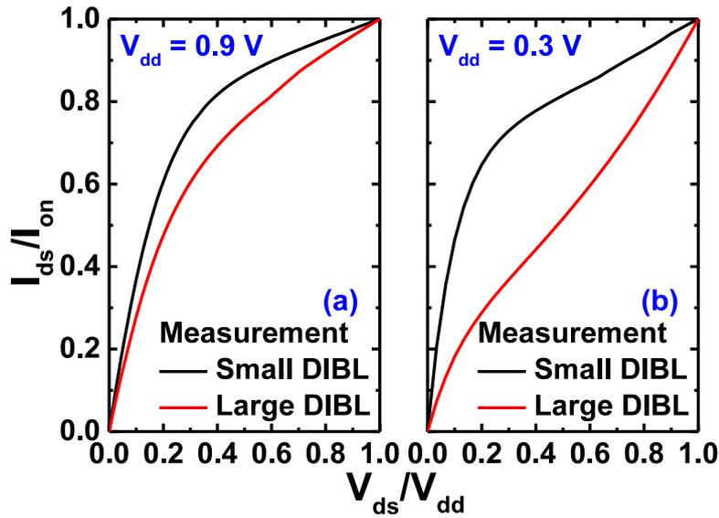
Figure 2.3 Normalized output curves of measured bulk nMOSFETs with DIBL in (a) above threshold region ( $V_{dd} = 0.9 \text{ V}$ ) and (b) subthreshold region ( $V_{dd} = 0.3 \text{ V}$ ). There is severe current degradation between small and large DIBL in subthreshold region.
