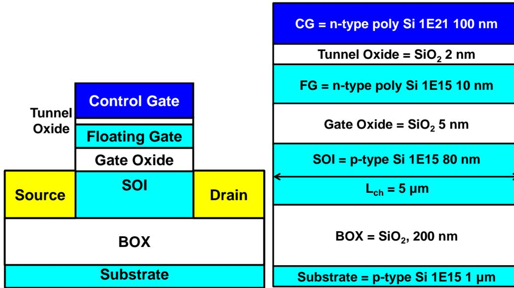
Figure 4.6 Schematic structure of simulated two-dimensional  $V_{th}$  self-adjusting MOSFET with FD-SOI.
