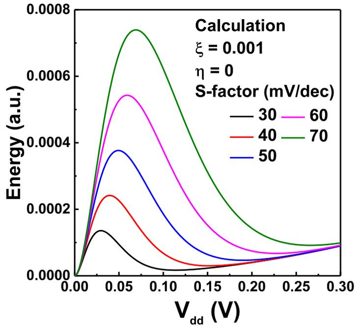
Figure 3.3 Calculated  $V_{dd}$  dependence of energy consumption with various s-factors when  $\eta$  factor is zero. The minima of  $V_{dd}$  and energy consumption decrease with steeper s-factor.
