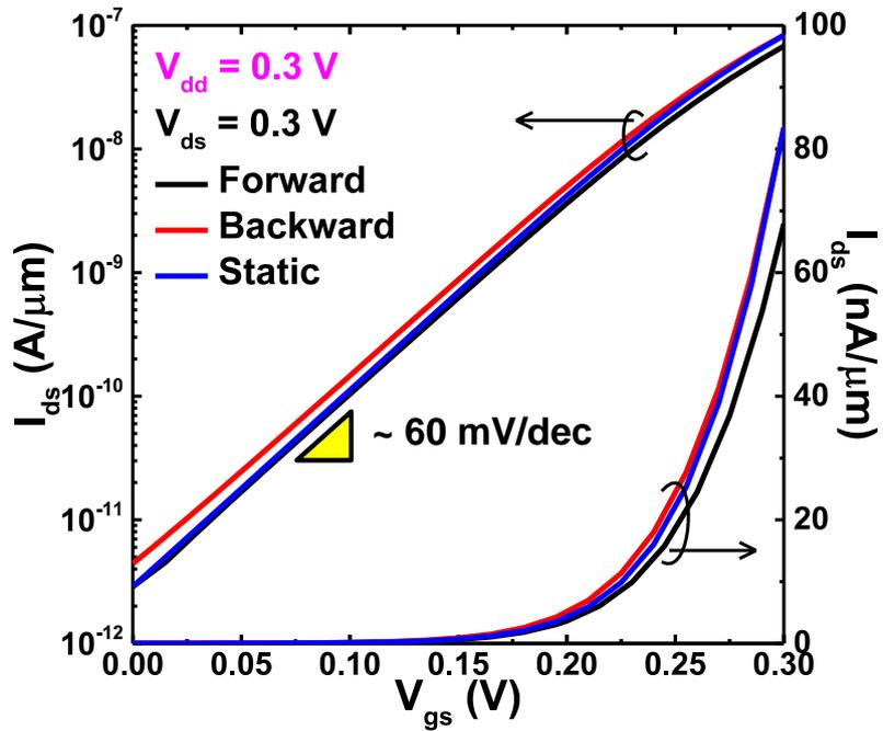
Figure 4.9 Simulated transfer curves of  $V_{th}$  self-adjusting MOSFET at  $V_{dd} = 0.3$  V.
