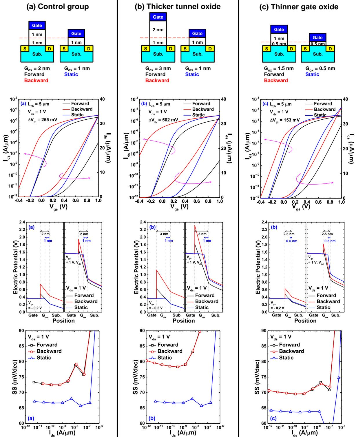
Figure 4.4 Simplified modeling structure and its transfer curves, electric potential and s-factor of  $V_{th}$  self-adjusting MOSFET at  $V_{dd} = 1$  V with (a) control group, (b) thicker tunnel oxide and (c) thinner gate oxide.
