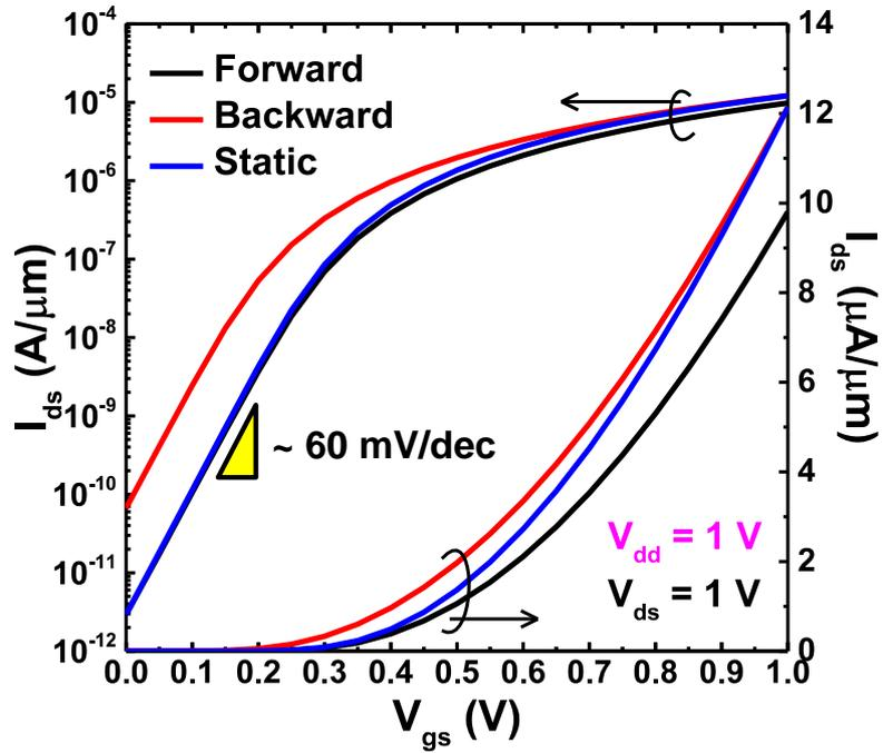
Figure 4.8 Simulated transfer curves of  $V_{th}$  self-adjusting MOSFET at  $V_{dd} = 1$  V.
