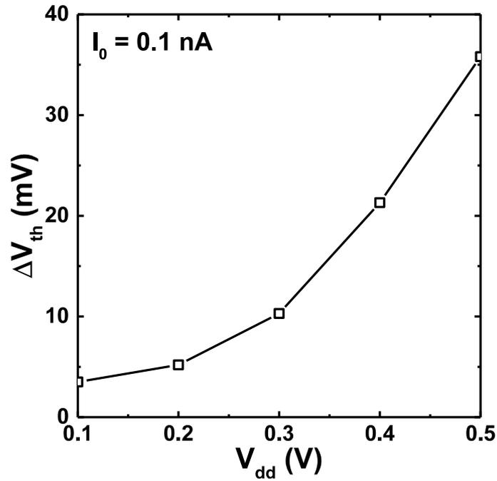
Figure 4.10 Extracted  $\Delta V_{th}$  with  $V_{dd}$  scaling.  $V_{th}$  self-adjusting characteristic is clearly shown even if  $\Delta V_{th}$  become smaller.
