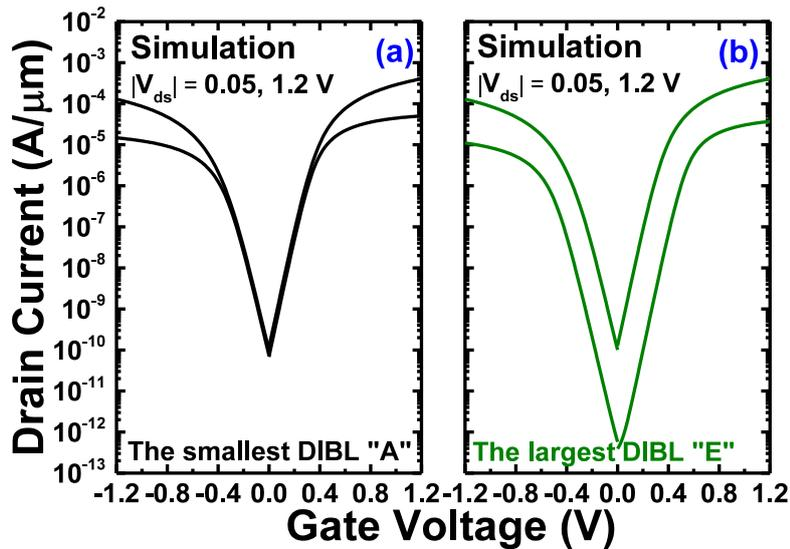
Figure 2.6 Simulated transfer curves of (a) the smallest DIBL device ‘A’ and (b) the largest DIBL device ‘E’.  $I_{on}$  and  $I_{off}$  is fixed at  $V_{gs} = V_{ds} = V_{dd}$  so that DIBL is reflected at  $V_{ds} = 0.05$  V
