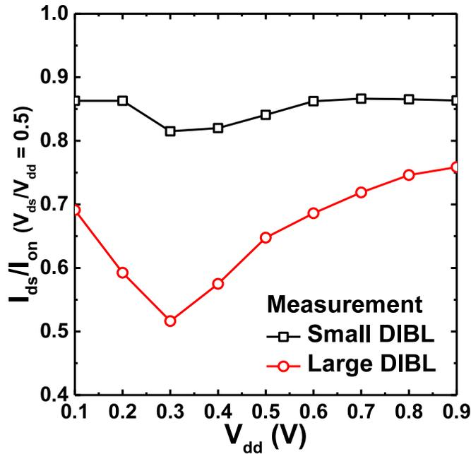
Figure 2.5 Normalized  $I_{ds}$  (at  $V_{ds}/V_{dd} = 0.5$ ) as a function of  $V_{dd}$  with small and large DIBL. Large DIBL device shows huge current degradation until at  $V_{dd} = 0.3$  V, subthreshold region.
