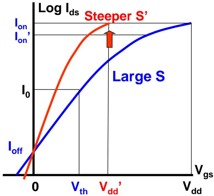
Figure 3.1 Transfer curves with large and steeper s-factor. Steeper s-factor leads to high performance with  $V_{dd}$  scaling.
