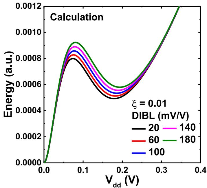
Figure 2.14 Calculated energy efficiency with various DIBL as a function of  $V_{dd}$ . The minimum points of energy consumption and  $V_{dd}$  become worse with DIBL increase.
