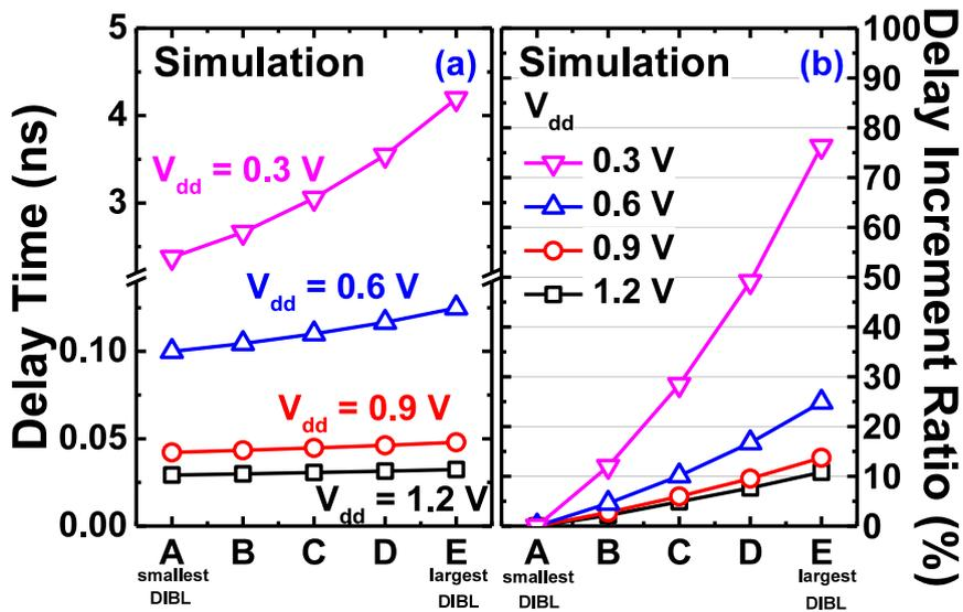
Figure 2.10 Delay time of CMOS ring oscillators with various  $V_{dd}$  and DIBL. The largest DIBL device 'E' in subthreshold region shows the slowest delay time.
