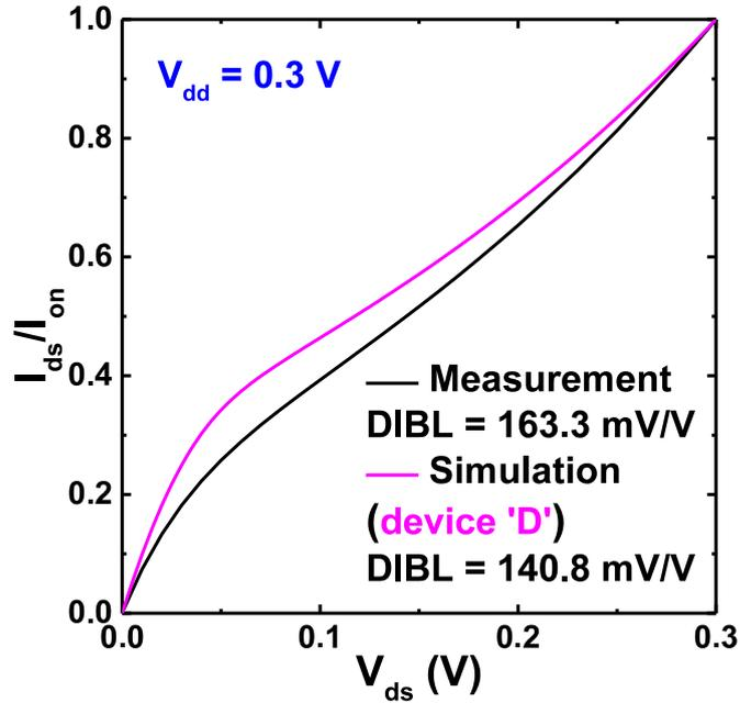
Figure 2.9 Comparison between normalized  $I_{ds}$  of measurement and simulation which have similar DIBL in subthreshold region. The simulation is well-matched with actual device.
