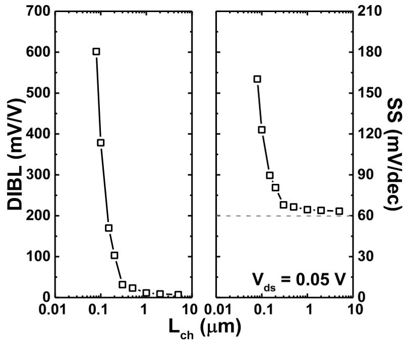
Figure 4.12 DIBL and s-factor with  $L_{ch}$  of  $V_{th}$  self-adjusting MOSFETs.
