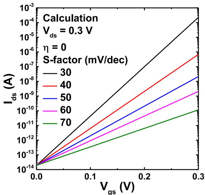
Figure 3.2 Calculated transfer curves with various s-factors.
