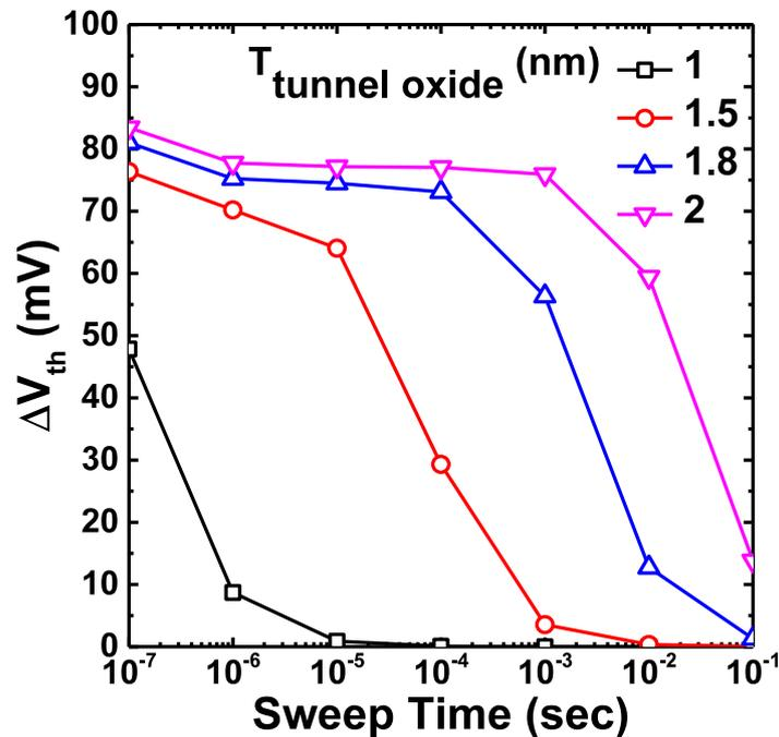
Figure 4.7  $\Delta V_{th}$  as a function of sweep time and tunnel oxide thickness. As the sweep time and tunnel oxide thickness is getting faster and thicker,  $\Delta V_{th}$  become larger.
