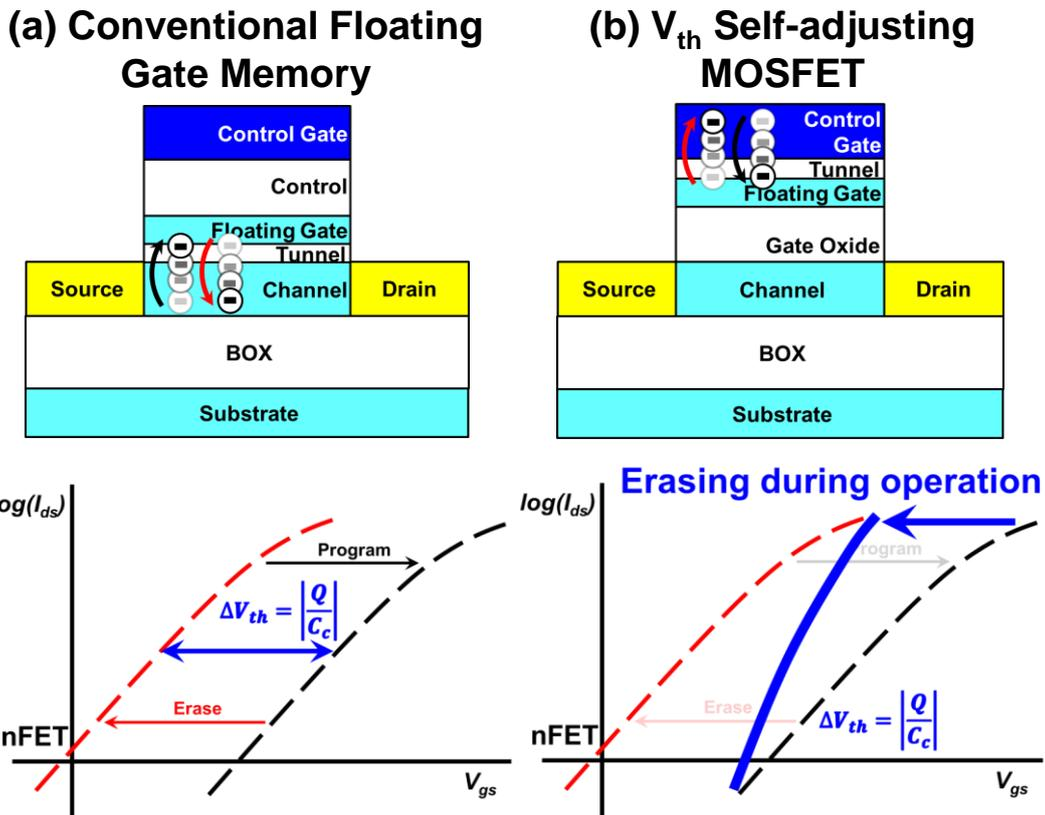
Figure 4.1 Schematic structure and transfer curves of (a) conventional floating gate memory and (b)  $V_{th}$  self-adjusting MOSFET. Note that thickness and location of tunnel oxide difference.
