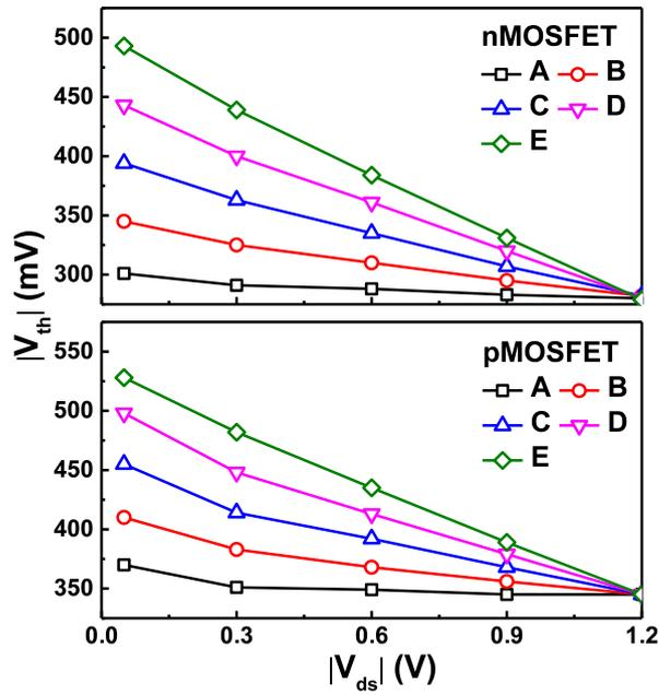
Figure 2.7  $V_{th}$  shift by various  $V_{ds}$  with simulated nMOSFETs and pMOSFETs.
