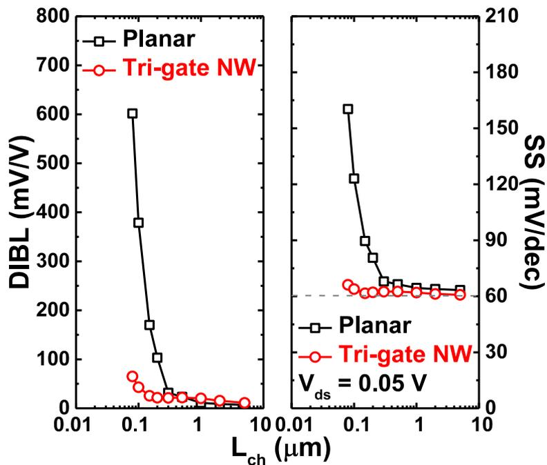
Figure 4.15 DIBL and s-factor with  $L_{ch}$  of planar and tri-gate nanowire structure. Tri-gate nanowire structure shows excellent immunity to short channel effects.
