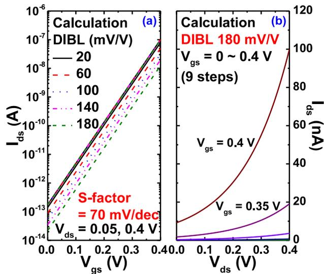
Figure 2.13 Calculated subthreshold current in (a) transfer curves with various DIBL and (b) output curves with DIBL value of 180 mV/V.
