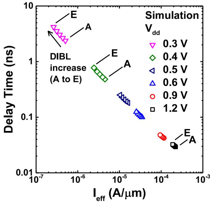
Figure 2.12 Correlation between delay time and  $I_{\text{eff}}$  with various  $V_{\text{dd}}$  and DIBL. Delay time and  $I_{\text{eff}}$  is degraded exponentially with  $V_{\text{dd}}$  scaling and becomes worse with DIBL increase.
