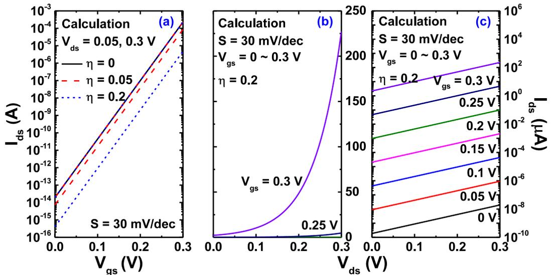
Figure 3.4 Calculated subthreshold current of steep s-factor as 30 mV/dec. (a) transfer curves with various  $\eta$  factors. (b), (c) linear and semi-log plot of output curves with  $\eta$  factor = 0.2, respectively.
