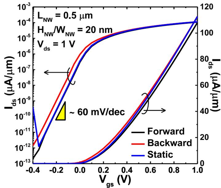
Figure 4.14 Simulated transfer curves of tri-gate nanowire MOSFET with  $V_{th}$  self-adjustment.
