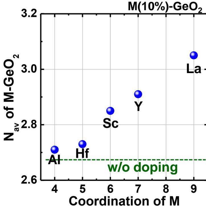
**Figure 2.21** Expected coordination numbers of M cation in GeO<sub>2</sub> network and the corresponding  $N_{av}$  of the total network.<sup>25, 26, 31</sup> Note that the M percentage here is controlled to be 10% for all the M-GeO<sub>2</sub>
