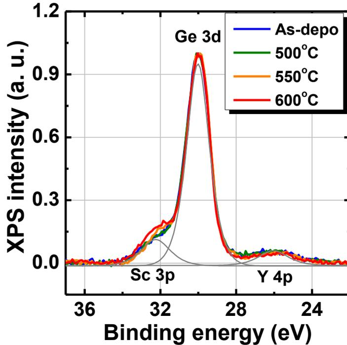
**Figure 3.12** XPS spectra from 4 nm  $\text{YScO}_3/\text{Ge}$  gate stacks. The spectra are de-convoluted into  $\text{Sc}3p$ ,  $\text{Y}4p$  and  $\text{Ge}3d$  peaks. Note that the spectra do not show obvious change with increasing the annealing temperature.
