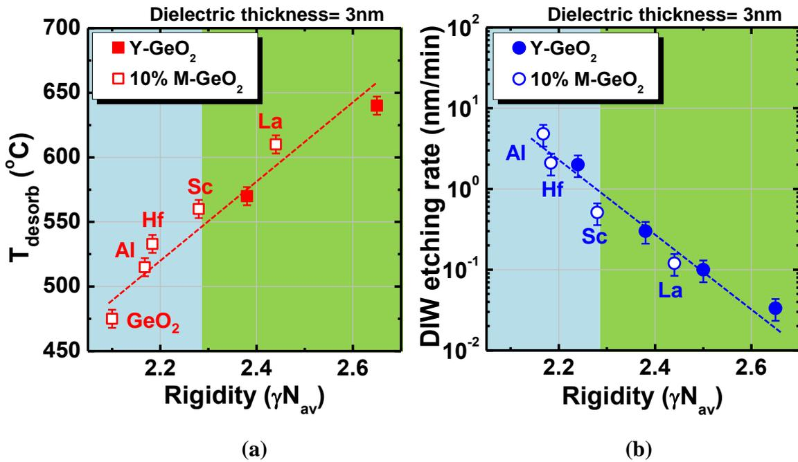
**Figure 2.22** (a)  $T_{\text{peak}}$  and (b)  $R_{\text{etching}}$  as a function of  $N_{\text{av}}$ . Note that the  $T_{\text{peak}}$  are from the M-GeO<sub>2</sub>/Ge and GeO<sub>2</sub>/Ge stack with the same thickness (3 nm). Here,  $\gamma$  is assumed to be 0.8 for all the materials in the figure.
