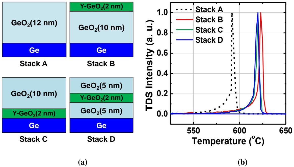
**Figure 2.8(a)** Schematic of bilayer stacks with top Y doping (10% Y-GeO<sub>2</sub>/GeO<sub>2</sub>/Ge), bottom Y doping (GeO<sub>2</sub>/10% Y-GeO<sub>2</sub>/Ge) and in the middle. (b) Corresponding GeO desorption spectra. The spectrum of a 12 nm Ge/GeO<sub>2</sub> stack is also shown as reference.
