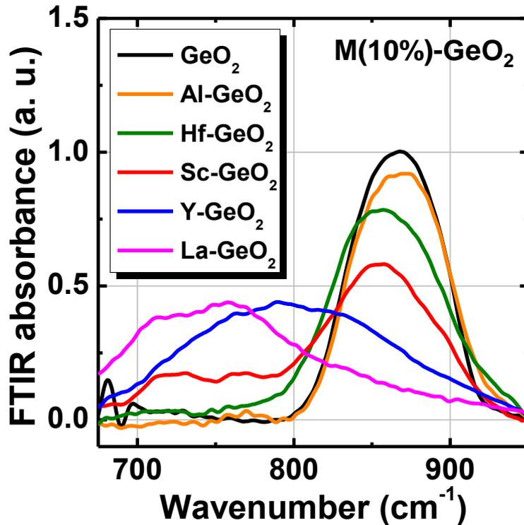
**Figure 2.23** FTIR absorbance spectra of M-GeO<sub>2</sub> and pure GeO<sub>2</sub>.<sup>12</sup> The peak shift of asymmetric stretching mode in GeO<sub>2</sub> to lower energy is clearly observed. The magnitude of this peak shift in different M-GeO<sub>2</sub> is an indication of how strongly the GeO<sub>2</sub> network is modified.
