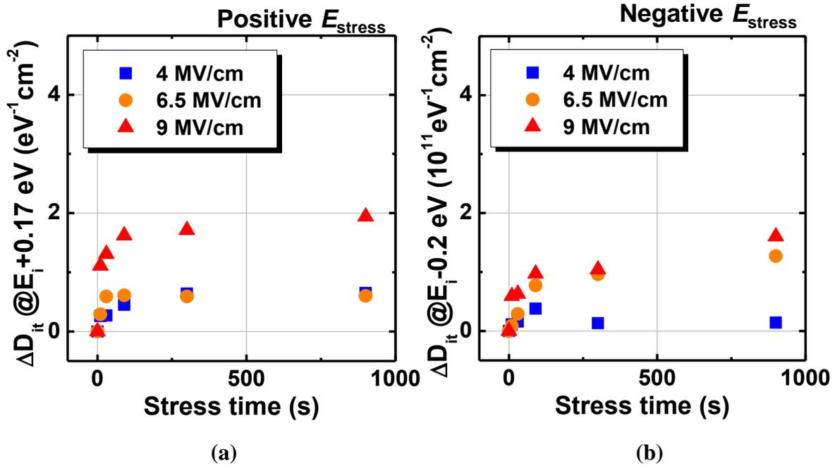
**Figure 4.19**  $D_{it}$  change in HPO-Y-GeO<sub>2</sub>/Ge stack as a function of stress time at various stress condition (4, 6.5 and 9 MV/cm of both polarities). The HPO-Y-GeO<sub>2</sub>/Ge is also the strongest gated stack against interface degradation among all the stacks reported in this work.
