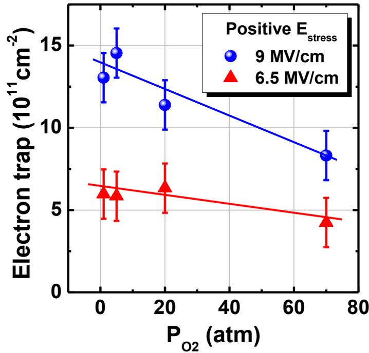
**Figure 4.9** The newly generated electron trap density in  $\text{GeO}_2/\text{Ge}$  stacks under positive  $E_{\text{stress}}$  as a function of  $P_{O_2}$  in the gate stack process. HPO can not sufficiently control the trap generation under high  $E_{\text{stress}}$  regardless of very promising properties in the initial and under low  $E_{\text{stress}}$  field.
