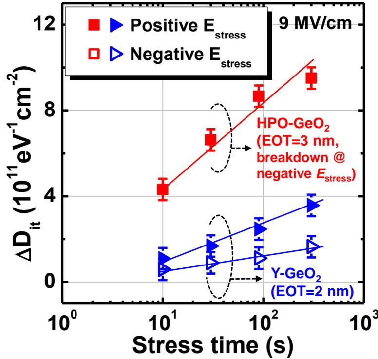
**Figure 4.13**  $D_{it}$  at  $V_{FB}$  ( $E_i-0.2$  eV or  $E_i+0.17$  eV for the p-Ge or n-Ge, respectively) increase in HPO-GeO<sub>2</sub> and Y-GeO<sub>2</sub>/Ge stacks as a function of time under positive or negative 9 MV/cm  $E_{stress}$ . Y-GeO<sub>2</sub> can suppress the  $D_{it}$  generation compared to that of HPO-GeO<sub>2</sub>.
