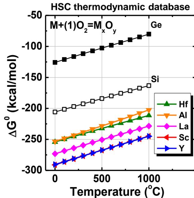
**Figure 2.3**  $\Delta G^0$  for various metal oxides formation as a function of temperature. Note that the reaction formulas are normalized to one O<sub>2</sub> molecule.
