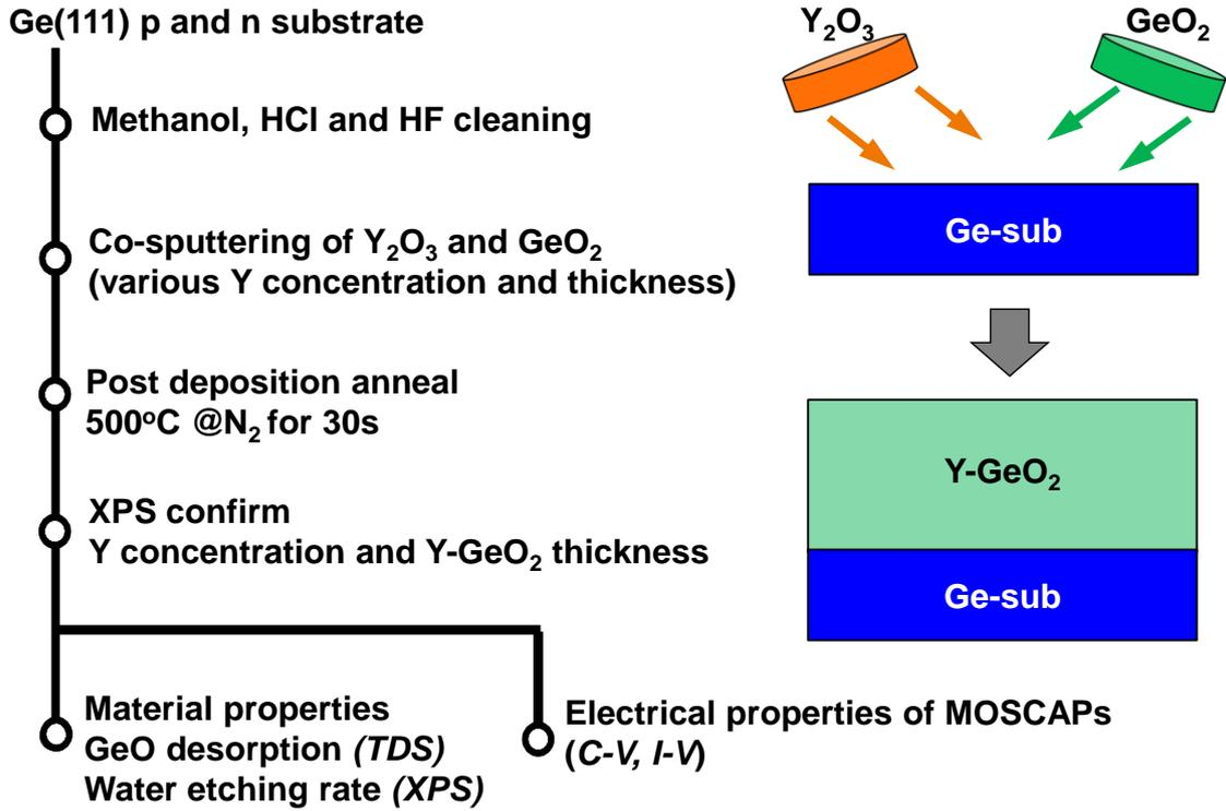
**Figure 2.4** Y-GeO<sub>2</sub>/Ge gate stack preparation process by rf co-sputtered technics. Note that the annealing process of this gate stack is pure N<sub>2</sub> ambient annealing in 1 atm pressure.
