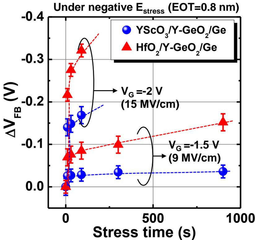
**Figure 4.21**  $V_{\text{FB}}$  shift in  $\text{HfO}_2/\text{Y-GeO}_2/\text{Ge}$  and  $\text{YScO}_3/\text{Y-GeO}_2/\text{Ge}$  stacks (EOT=0.8 nm) as a function of time under high negative  $V_{\text{G}}$  ( $V_{\text{G}}=1.5$  and  $2$  V,  $E_{\text{stress}}=10$  and  $15$  MV/cm). The  $\text{YScO}_3/\text{Y-GeO}_2/\text{Ge}$  stacks show less  $V_{\text{FB}}$  shift than the  $\text{HfO}_2$  counterpart at a fixed  $V_{\text{G}}$  and EOT.
