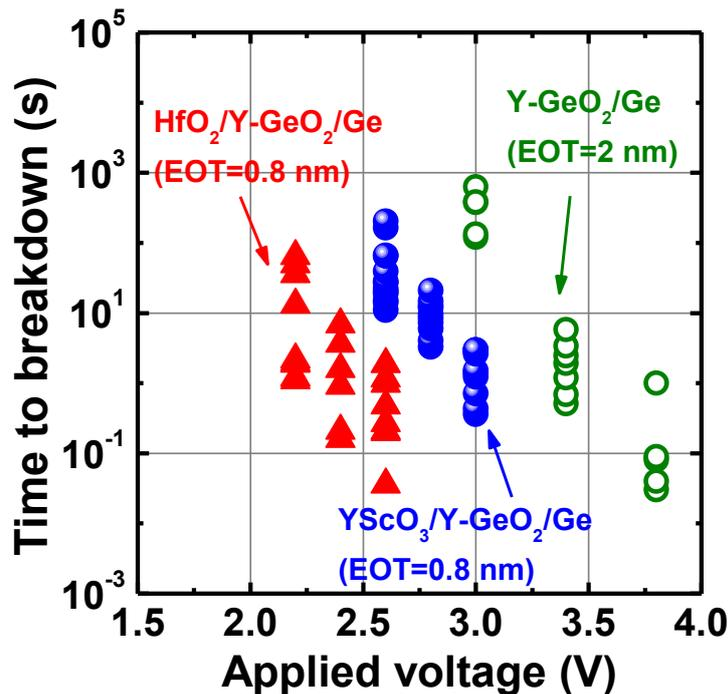
**Figure 4.23** Time to breakdown as a function of  $E_{\text{stress}}$  in  $\text{YScO}_3/\text{Y-GeO}_2/\text{Ge}$  (EOT 0.8 nm),  $\text{HfO}_2/\text{Y-GeO}_2/\text{Ge}$  (EOT 0.8 nm) and  $\text{Y-GeO}_2/\text{Ge}$  (EOT 2 nm) stacks.
