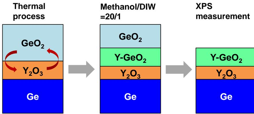
**Figure 3.3** Experimental procedures to estimate the intermixing thickness at the  $\text{GeO}_2/\text{Y}_2\text{O}_3$  interface. The critical point here is the different DIW etching rate between the intermixed layer and pure  $\text{GeO}_2$ .
