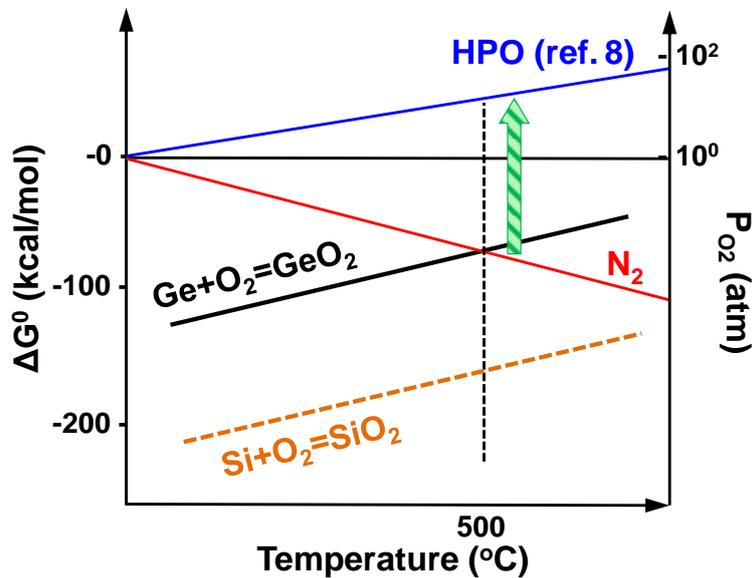
**Figure 2.2** Ellingham diagram for GeO<sub>2</sub> and SiO<sub>2</sub> formation under various oxygen ambient conditions calculated from thermodynamic data base.<sup>7</sup>
