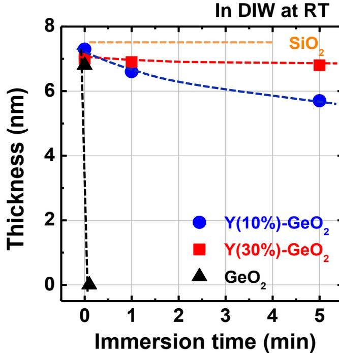
**Figure 2.10** Thickness of Y-GeO<sub>2</sub> and GeO<sub>2</sub> as a function of immersion time in pure DIW. The solubility of Y-GeO<sub>2</sub> is drastically decreased.<sup>14</sup> Note that SiO<sub>2</sub> is insoluble in water.
