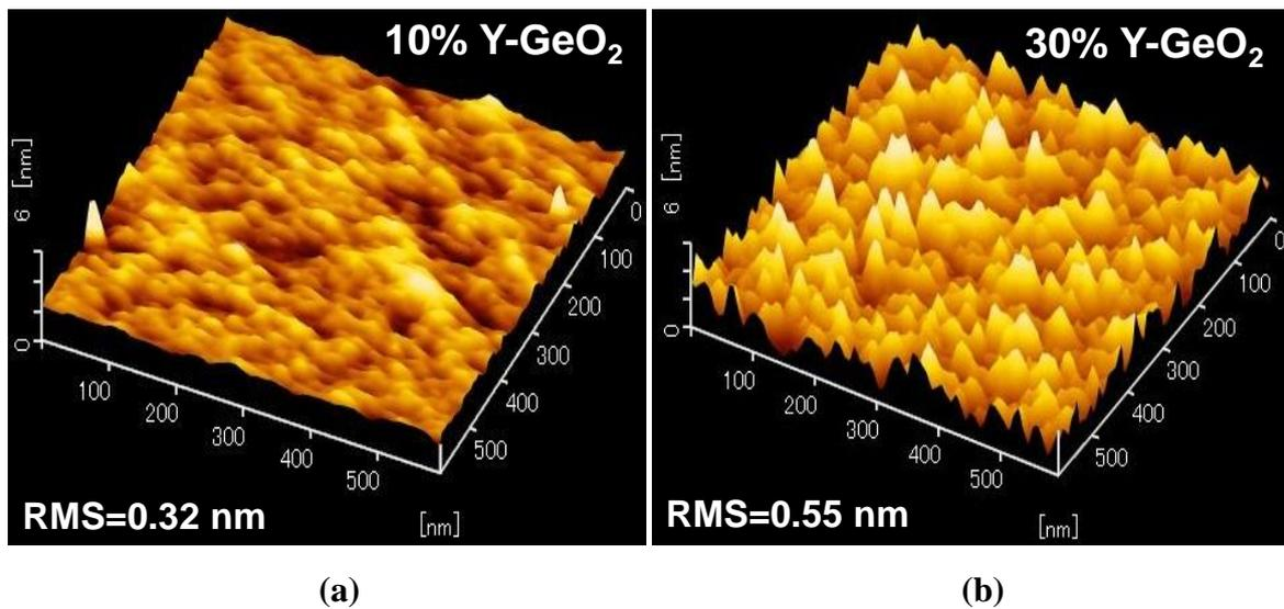
**Figure 2.29** AFM images of the top surface of (a) 10% Y-GeO<sub>2</sub> and (b) 30% Y-GeO<sub>2</sub> after 5 min immersion in DIW. The 10% Y-GeO<sub>2</sub> is uniformly etched by water, while 30% Y-GeO<sub>2</sub> shows some localized particles.
