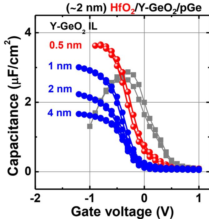
**Figure 3.5** Bidirectional  $C$ - $V$  curves of  $\text{HfO}_2/\text{Y-GeO}_2/\text{Ge}$  stacks with various  $\text{Y-GeO}_2$  IL thicknesses measured at RT. It is notable that decent  $C$ - $V$  curves are kept with  $\text{Y-GeO}_2$  thickness over 1 nm, while thinner  $\text{Y-GeO}_2$  thickness (below 1 nm) results in the degradation of the  $C$ - $V$  curve. The  $\text{HfO}_2/(1 \text{ nm}) \text{ GeO}_2/\text{Ge}$  stack also shows poor electrical properties.
