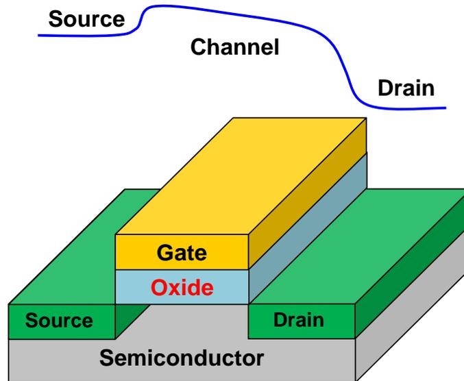
**Figure 1.1** Schematics of a MOSFET with planar structure. There are three terminals for the device, the source, the drain and the gate. The carriers are injected from the source to the drain through the semiconductor channel, which is controlled by field applied through gate electrode.
