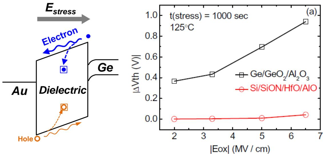
**Figure 1.10(a)** Schematics of the carrier trapping in Ge MOS device under and positive  $E_{stress}$ . The electrons are injected from the Ge to gate metal and the holes are injected in an inverse direction. Both might be captured by the trap sites in the dielectric. Similar situation can be expected for negative  $E_{stress}$ . **(b)**  $V_{th}$  shift as a function of electric field in Ge and Si stacks.<sup>50</sup>
