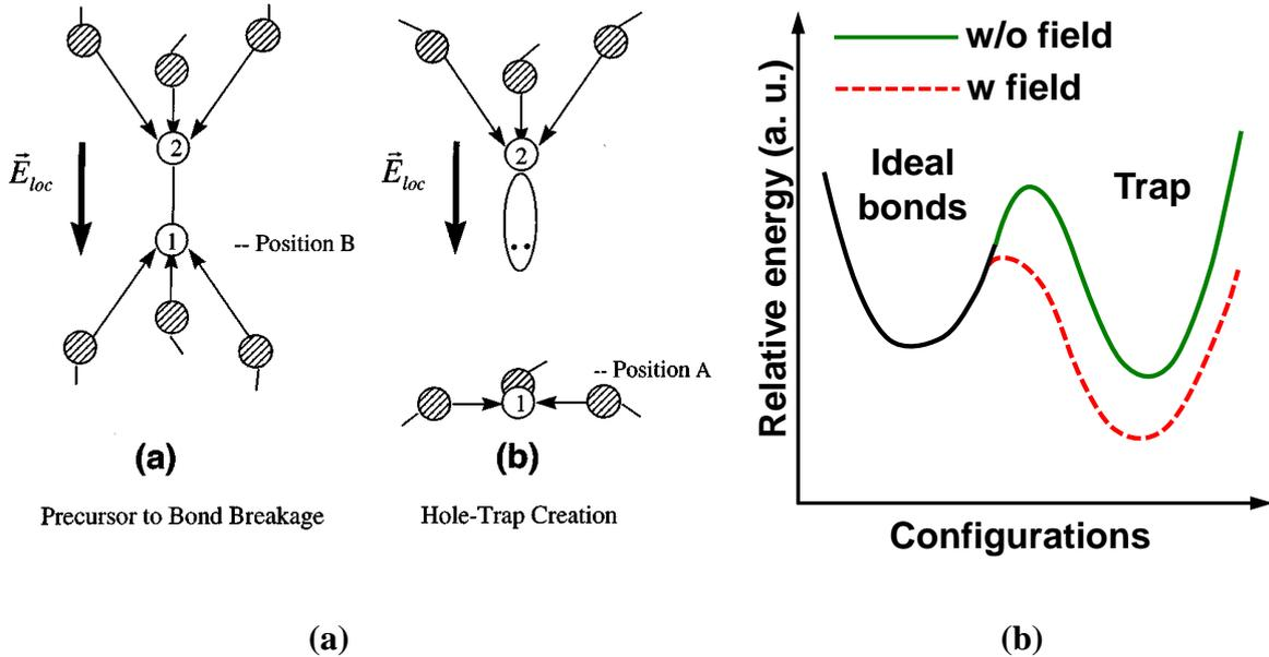
**Figure 4.4(a)** Atomistic schematics of thermochemical model for dielectric degradation in  $\text{SiO}_2$ .<sup>18, 20</sup> The chemical bonds in the dielectric are broken by the  $E_{loc}$  (dependent on the dielectric thickness,  $V_G$  and  $k$ -value) and the ions are displaced from the original sites, which results in the generation of hole traps. **(b)** Schematically shows the energy states corresponding to the ideal dielectric and trap generation with and without electric field.
