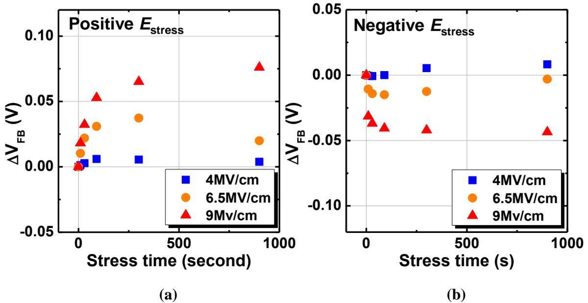
**Figure 4.17**  $V_{FB}$  shift in HPO-Y-GeO<sub>2</sub>/Ge stack as a function of stress time at various stress condition (4, 6.5 and 9 MV/cm of (a) positive and (b) negative  $E_{stress}$ ). It is worth noting that the  $V_{FB}$  shift in this gate stack is the smallest among all the gates stacks discussed in this chapter.
