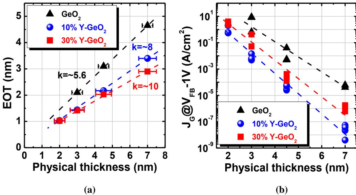
**Figure 2.13(a)** EOT as a function of Y-GeO<sub>2</sub> and GeO<sub>2</sub> physical thickness. It is notable that the enhancement of  $k$ -value is observed by Y-doping in GeO<sub>2</sub>.<sup>14</sup> **(b)**  $J_G$  as a function of Y-GeO<sub>2</sub> and GeO<sub>2</sub> physical thickness.<sup>14</sup>
