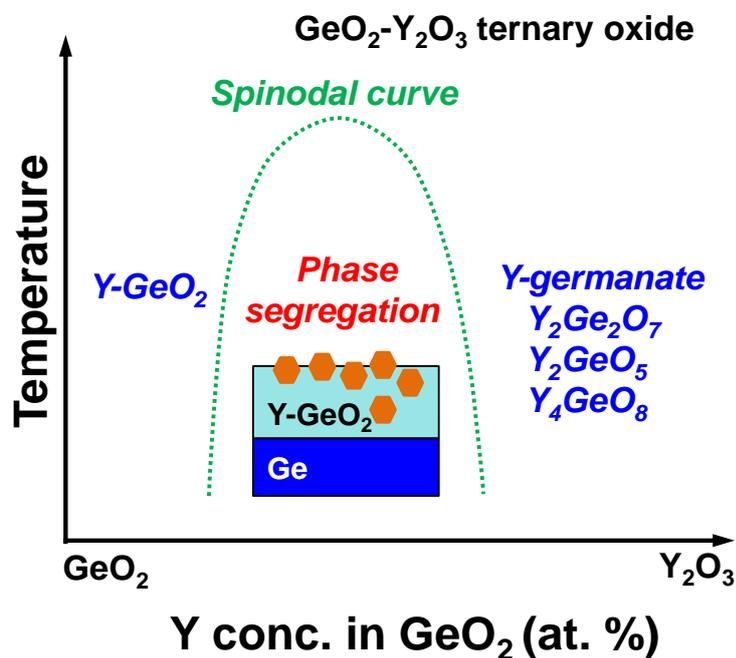
**Figure 2.30** Phase diagram of GeO<sub>2</sub>-Y<sub>2</sub>O<sub>3</sub> ternary oxide.<sup>41</sup> Mainly three regions exist in the diagram, namely, Y-GeO<sub>2</sub>, Y-rich germanate and phase segregation region.
