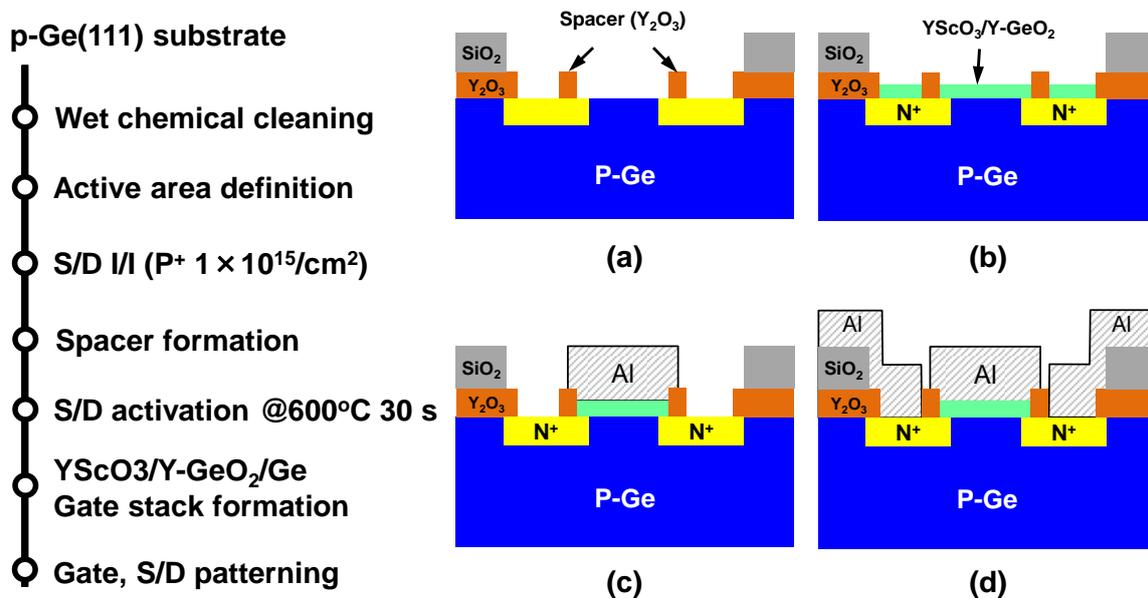
**Figure 3.15** Process flow and schematics of Ge n-MOSFET with YScO<sub>3</sub>/Y-GeO<sub>2</sub>/Ge gate stacks. 30 nm Y<sub>2</sub>O<sub>3</sub> and 500 nm SiO<sub>2</sub> were deposited to form the spacer and field oxides,
