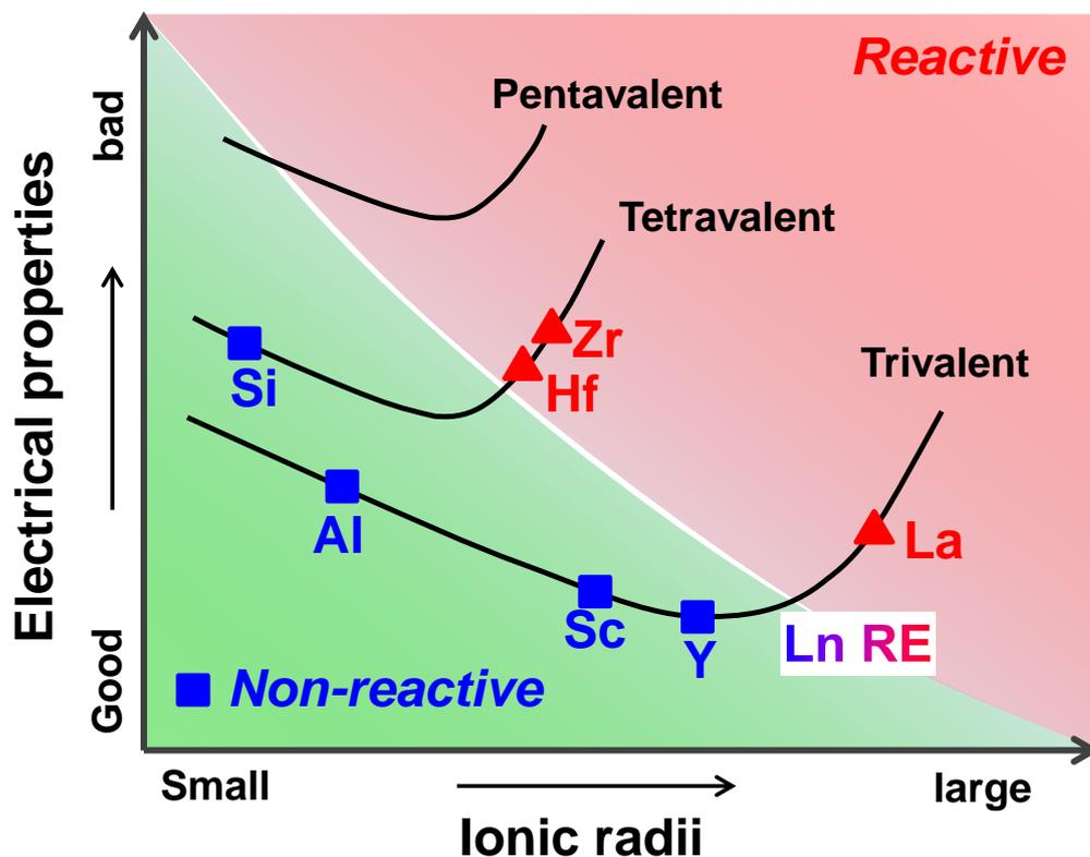
**Figure 2.31.** Schematic of two semi-empirical criteria for the interface properties in different M-GeO<sub>2</sub>/Ge stack. The doping species that are reactive with Ge substrate are in the red region and the unreactive ones are in the blue region. Note that part of the Ln RE cations are reactive with Ge.
