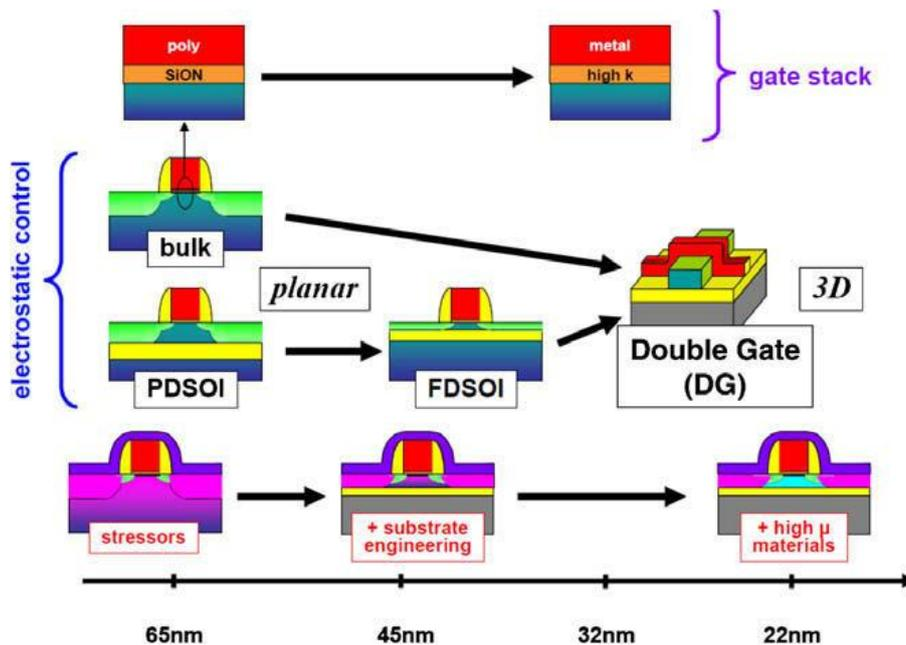
**Figure 1.3** Schematics of various approaches to improve the device properties in the post dimensional scaling age.<sup>13</sup> The device structure, gate insulator material and channel material are all possible components that can be improved.
