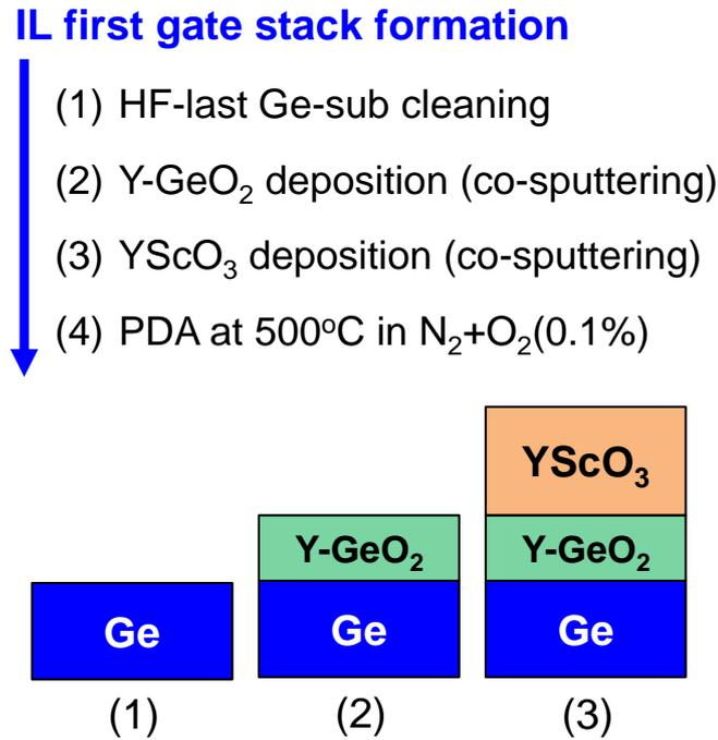
**Figure 3.6** Schematics of  $\text{YScO}_3/\text{Y-GeO}_2/\text{Ge}$  gate stack process. Note that in the step 3, low sputtering power is preferred to reduce damage to the passivated interface.
