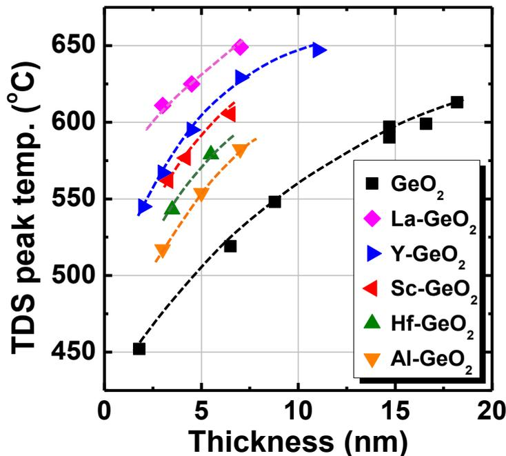
**Figure 2.19** TDS peak temperature of GeO desorption as a function of initial M-GeO<sub>2</sub> and GeO<sub>2</sub> thickness.<sup>12</sup> The improvements of the thermal stability by different metal oxides doping, from lowest to highest, are in the order of Al<sub>2</sub>O<sub>3</sub>, HfO<sub>2</sub>, Sc<sub>2</sub>O<sub>3</sub>, Y<sub>2</sub>O<sub>3</sub> and La<sub>2</sub>O<sub>3</sub>.
