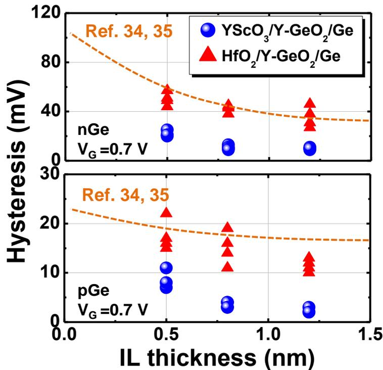
**Figure 4.20** Hysteresis of the  $C-V$  curves in  $\text{HfO}_2/\text{Y-GeO}_2/\text{Ge}$  and  $\text{YScO}_3/\text{Y-GeO}_2/\text{Ge}$  stacks as a function of  $\text{Y-GeO}_2$  IL thickness. The references show the hysteresis of the Ge gate capacitances with  $\text{GeO}_x$  as IL.<sup>34, 35</sup>
