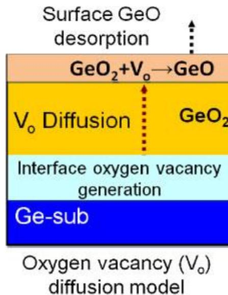
**Figure 2.1** schematics of GeO desorption mechanism in GeO<sub>2</sub>/Ge stacks under thermal process.<sup>2</sup> The GeO desorption process is accompanied by the  $\text{V}_o$  formation and diffusion throughout the GeO<sub>2</sub> layer, which result in drastic degradation of electrical properties.
