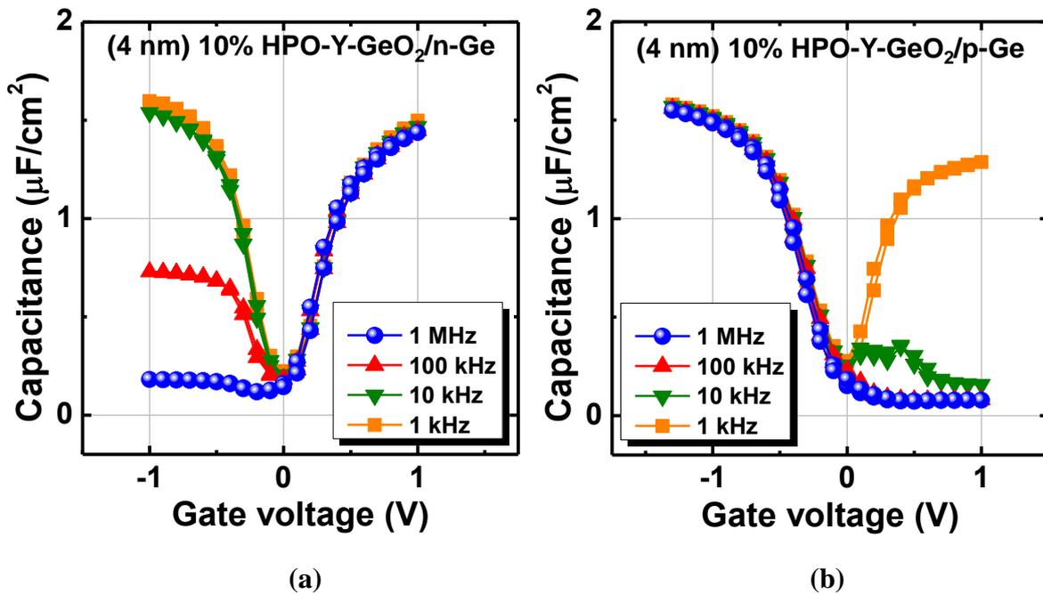
**Figure 4.16** (a) Bidirectional  $C$ - $V$  curves of an Au/10% HPO-Y-GeO<sub>2</sub>/n-Ge MOSCAPs measured at RT. (b) Bidirectional  $C$ - $V$  curves of Au/10% HPO-Y-GeO<sub>2</sub>/p-Ge MOSCAPs.
