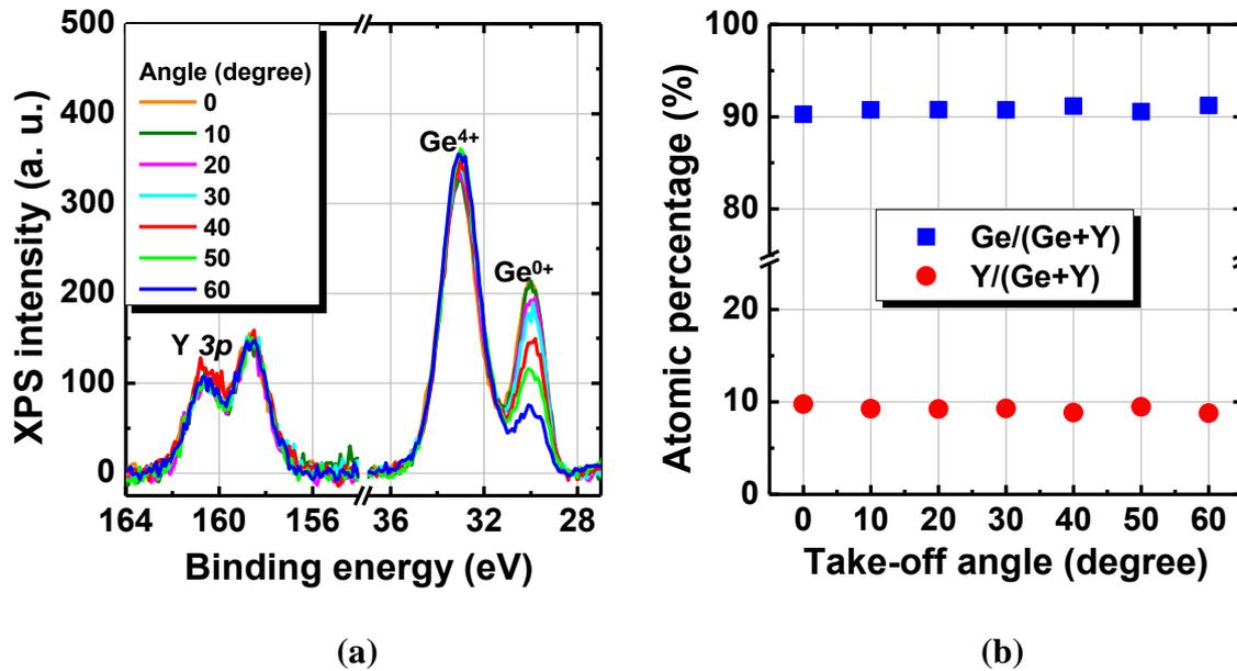
**Figure 2.6** (a) Angle-resolved XPS spectra of Y-GeO<sub>2</sub>/Ge stack. The intensity ratio between Ge 3d<sup>4+</sup> and Y 3p is not changed by changing the take-off angle. (b) The atomic percentage of Y and Ge among metallic atoms calculated from the XPS spectra as a function of take-off angle.
