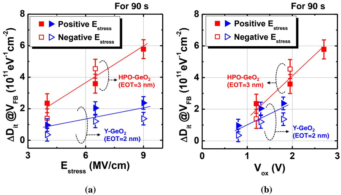
**Figure 4.14**  $D_{it}$  at  $V_{FB}$  increase after 90 sec stress for HPO-GeO<sub>2</sub> and Y-GeO<sub>2</sub>/Ge stacks as a function of (a)  $E_{stress}$  and (b)  $V_{OX}$ . The  $V_{FB}$  here is  $E_i - 0.2$  eV or  $E_i + 0.17$  eV for the p-Ge or n-Ge, respectively. Regardless of the X-axis, the smaller  $D_{it}$  generation in Y-GeO<sub>2</sub>/Ge stack can be confirmed in the viewpoint of both  $E_{stress}$  and  $V_{OX}$ .
