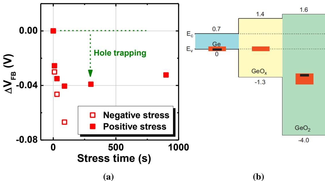
**Figure 4.6(a)**  $V_{FB}$  shift in 1 atm  $\text{GeO}_2/\text{Ge}$  stacks under 4 MV/cm  $E_{\text{stress}}$  with both polarities. The large negative shift of the  $V_{FB}$  represents the large amount of hole trapping. **(b)** The
