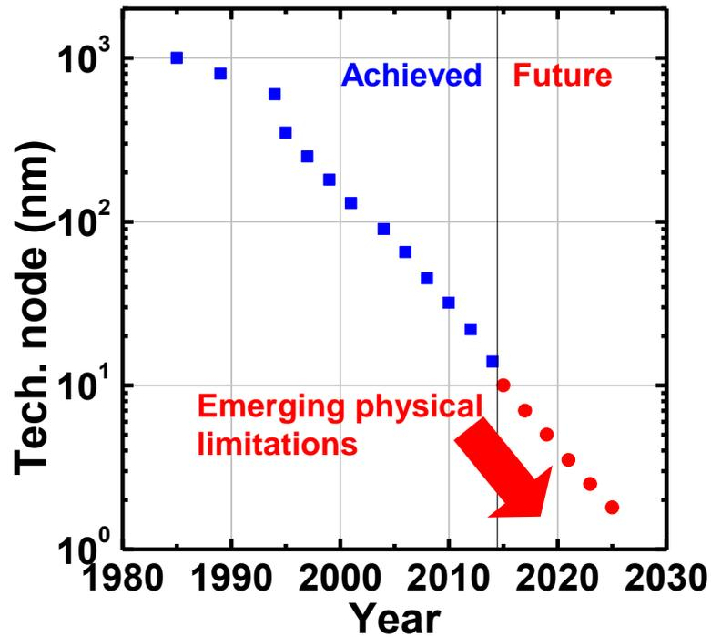
**Figure 1.2** ITRS technology node of device scaling by years.<sup>15</sup> The half reduction of the device dimensions has been successfully carried out every 3 years so far, but further reducing the device size to a few nm will inevitably face the physical limitations.
