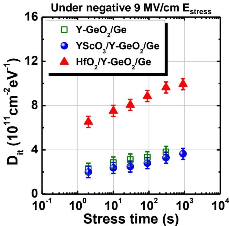
**Figure 4.22**  $D_{it}$  at  $E_i-0.2$  eV of  $\text{YScO}_3/\text{Y-GeO}_2/\text{Ge}$  and  $\text{HfO}_2/\text{Y-GeO}_2/\text{Ge}$  gate stacks as a function of time under 9 MV/cm negative  $E_{\text{stress}}$ . The  $D_{it}$  at  $\text{Y-GeO}_2/\text{Ge}$  stack is also shown for comparison.
