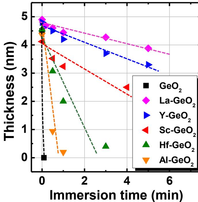
**Figure 2.20** Thicknesses of M-GeO<sub>2</sub> and pure GeO<sub>2</sub> estimated from XPS as a function of immersion time in DIW.<sup>12</sup> The water resistance increase by different metal oxides doping, from weakest to strongest, is Al, Hf, Sc, Y and La.
