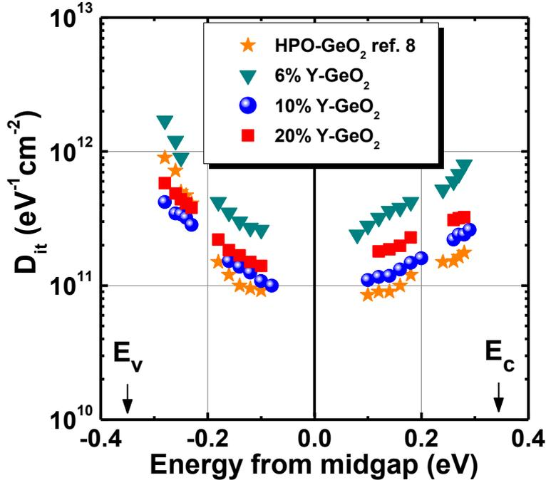
**Figure 2.12** Energy distribution of the estimated  $D_{it}$  in the Au/Y-GeO<sub>2</sub>/Ge stacks with various Y percentages measured by low-temperature conductance method. The state of art low  $D_{it}$  at GeO<sub>2</sub>/Ge interface prepared by HPO is also shown for comparison.<sup>8</sup>
