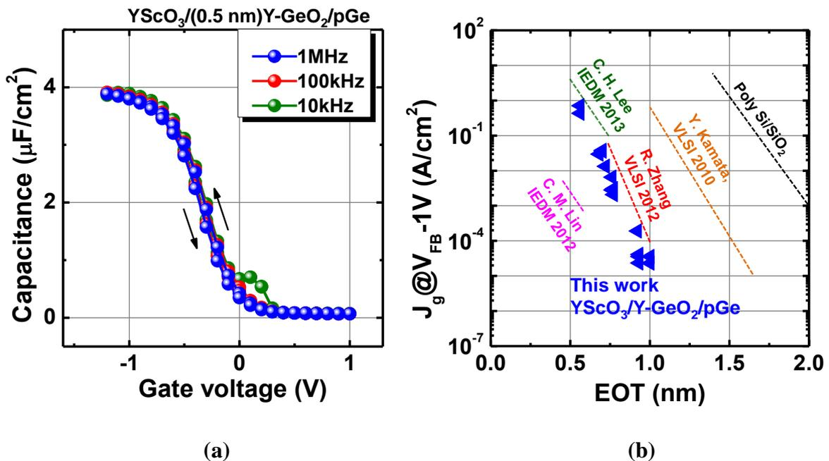
**Figure 3.14(a)** Bidirectional  $C$ - $V$  curves of  $\text{YScO}_3/(0.5 \text{ nm})\text{Y-GeO}_2/\text{Ge}$  gate stacks with EOT about 0.5 nm measured at RT.<sup>24</sup> No hysteresis and frequency dispersion in  $C$ - $V$  curves
