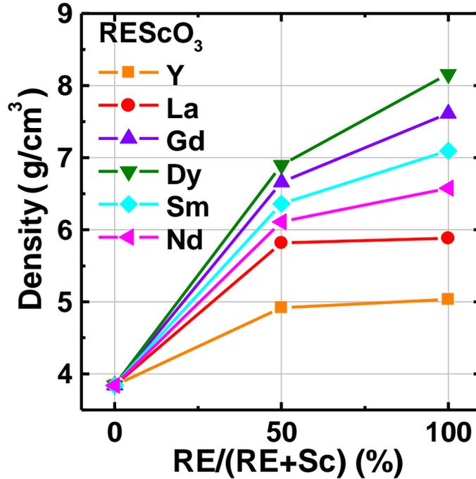
**Figure 3.10** Densities of some  $\text{REScO}_3$  and that of their binary compounds. Note that the densities of  $\text{REScO}_3$  are higher than linear combination of their binary compounds, which indicates that they are more densely packed.
