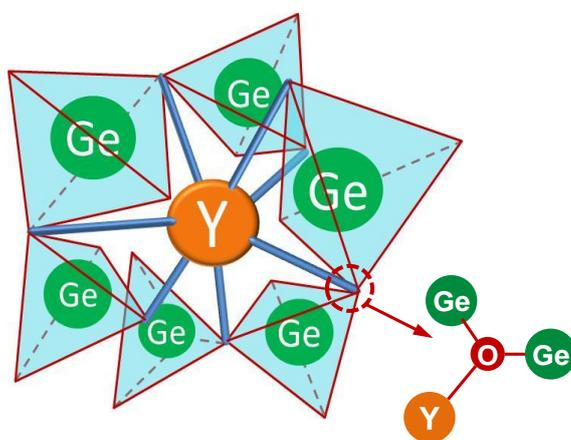
**Figure 2.16** Schematics of MRN structure of Y-GeO<sub>2</sub>. Due to the large amount of additional Y-O bond, some O atoms increase their coordination to 3 as well.
