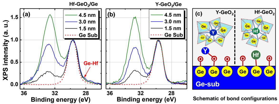
**Figure 2.26** Ge<sub>3d</sub> core level spectra of (a) Hf-GeO<sub>2</sub>/Ge and (b) Y-GeO<sub>2</sub>/Ge measured by XPS,<sup>12</sup> Note that the spectrum of the as-cleaned Ge substrate is also shown in the dotted line for comparison. The Ge-Hf metallic bond is preferentially observed in Hf-GeO<sub>2</sub>/Ge stack. (c) Schematic of the bond configurations in Y-GeO<sub>2</sub>/Ge and Hf-GeO<sub>2</sub>/Ge stacks.<sup>12</sup>
