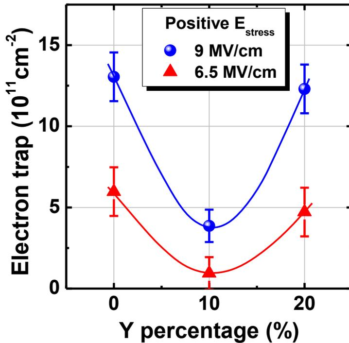
**Figure 4.10** The newly generated electron trap density in Y-GeO<sub>2</sub>/Ge stacks as a function of Y percentage under positive  $E_{\text{stress}}$ . Small amount of Y doping can drastically suppress the trap generation while high Y percentage degrades it again.
