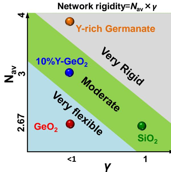
**Figure 2.17** Network rigidity as a function of  $N_{av}$  estimated from the structures of Y-GeO<sub>2</sub> and GeO<sub>2</sub>.<sup>29</sup> The better rigidity of Y-GeO<sub>2</sub> than the flexible GeO<sub>2</sub> network results in its both better thermal stability and water resistance. Note that the  $\gamma$  value is assumed to be 0.8 here for all the GeO<sub>2</sub> based oxides ( $\gamma=1$  for SiO<sub>2</sub>).
