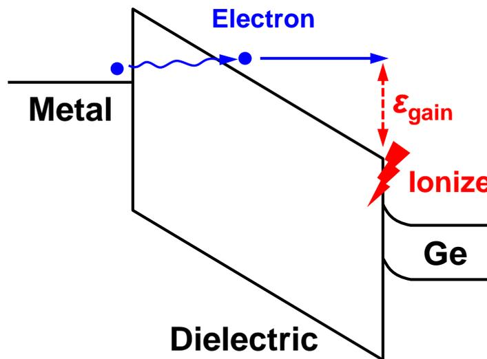
**Figure 4.3** Schematic of carrier injection model for trap generation in the dielectrics under a negative  $E_{\text{stress}}$ .<sup>17</sup> The electrons from the gate metal are accelerated by the external electric field and acquire the sufficient  $\epsilon_{\text{gain}}$  to break the bond near interface. For the positive  $E_{\text{stress}}$ , similar mechanism is involved except for that the holes are generated by the injected electrons.
