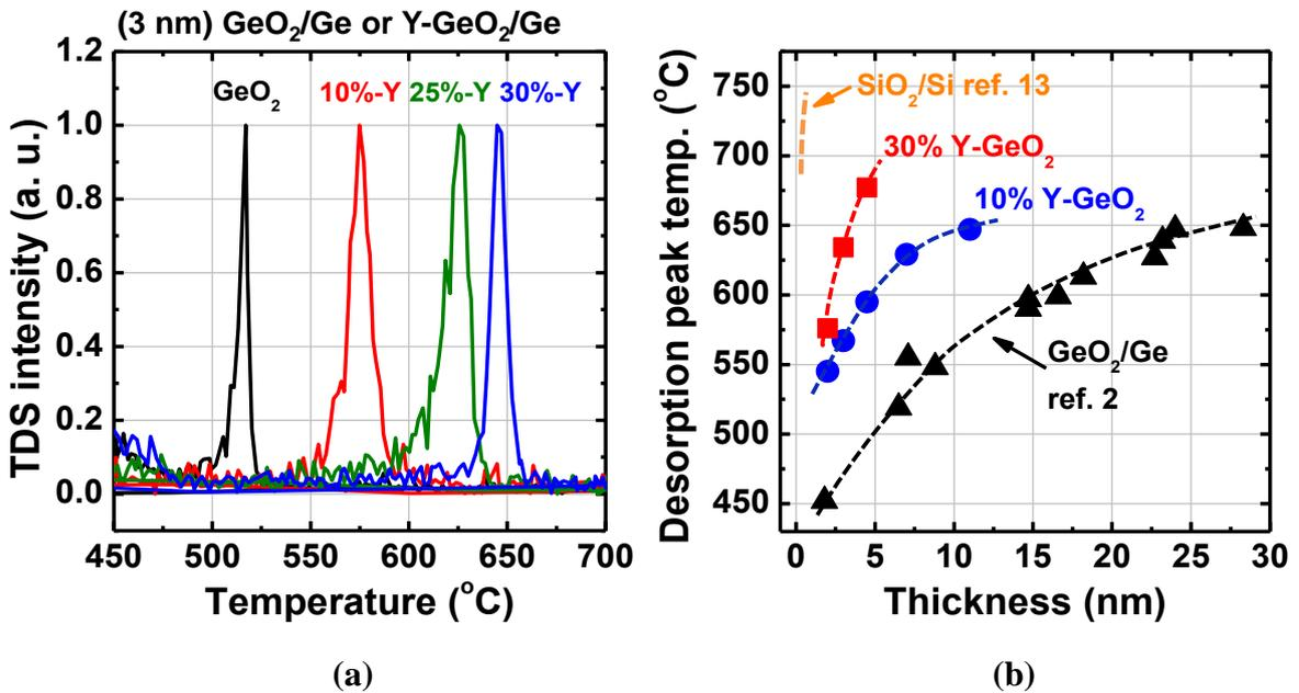
**Figure 2.7(a)** TDS spectra corresponding GeO ( $m/z=90$ ) from Y-GeO<sub>2</sub>/Ge and pure GeO<sub>2</sub>/Ge stacks. Note that the thicknesses of the dielectrics are 3 nm in these stacks. **(b)**
