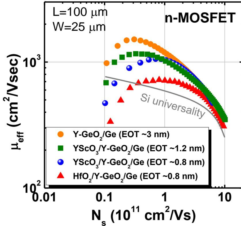
**Figure 3.16** The  $\mu_{\text{eff}}$  of YScO<sub>3</sub>/Y-GeO<sub>2</sub>/Ge n-MOSFETs where the Y-GeO<sub>2</sub> IL thickness is fixed at 1 nm. The  $\mu_{\text{eff}}$  in the Y-GeO<sub>2</sub>/Ge n-MOSFET is also shown for comparison<sup>5</sup>. The peak  $\mu_{\text{eff}}$  of 1057cm<sup>2</sup>/Vsec with EOT 0.8 nm is demonstrated in YScO<sub>3</sub>/Y-GeO<sub>2</sub>/Ge, which is the highest one in sub-nm EOT region due to the immunity to interface degradation.
