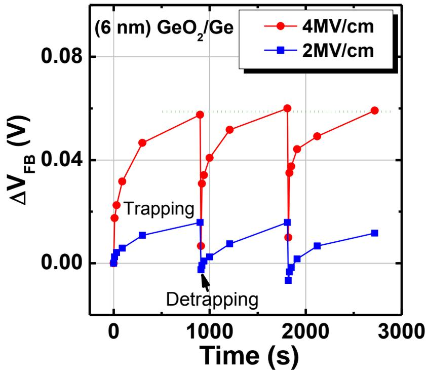
**Figure 4.8**  $V_{FB}$  shift under circularly trapping-detrapping process by 900 sec of positive  $E_{stress}$  and 10 sec of negative  $E_{stress}$ . It is found that the trapping is highly repeatable under both 2 and 4 MV/cm, which indicate that the trap generation can be neglected in these stress condition.
