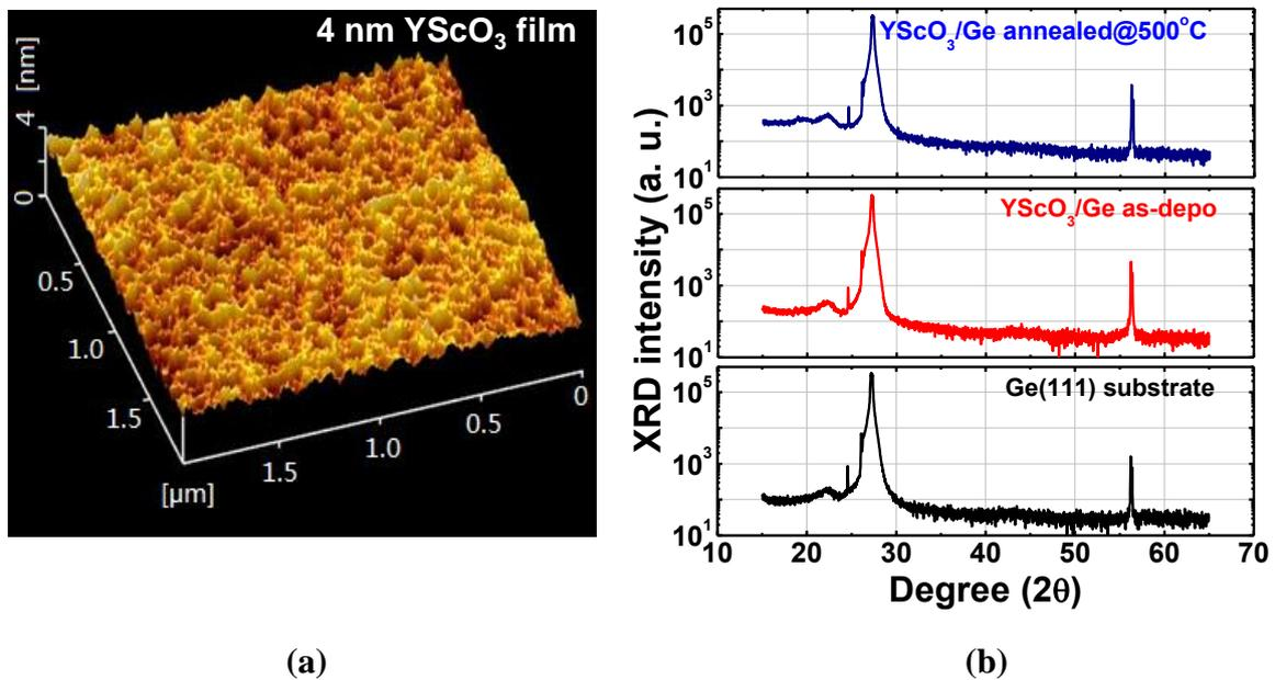
**Figure 3.7(a)** AFM image of the top surface of 4 nm YScO<sub>3</sub>/Ge stack after annealing. The RMS roughness is about 0.3 nm. **(b)** XDR pattern of (40 nm) YScO<sub>2</sub>/Ge gate stacks (both annealed and as-deposited). The XRD pattern of Ge(111) substrate are also shown for comparison.
