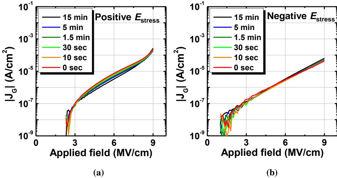
**Figure 4.18**  $J_G$  (absolute value) in HPO-Y-GeO<sub>2</sub>/Ge gate stack with different stress time at 9 MV/cm. The low initial  $J_G$  reflects that HPO-Y-GeO<sub>2</sub>/Ge is an initially ideal gate dielectric. While the negligible SILC in this gate stack indicates its remarkably strong ability against trap generation.
