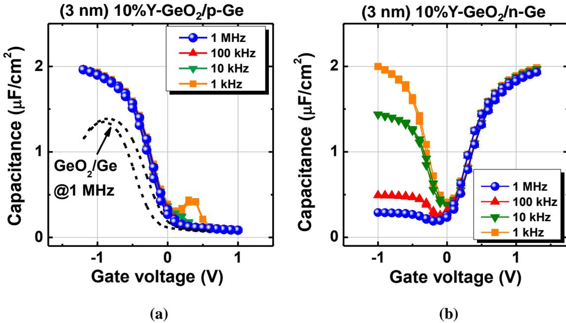
**Figure 2.11** (a) Bidirectional  $C$ - $V$  curves of an Au/10% Y-GeO<sub>2</sub>/p-Ge MOSCAPs measured at RT. The 1 MHz  $C$ - $V$  curve of a sputtered (3nm) GeO<sub>2</sub>/p-Ge stack is also shown for comparison. (b) Bidirectional  $C$ - $V$  curves of Au/10% Y-GeO<sub>2</sub>/n-Ge MOSCAPs measured at RT.
