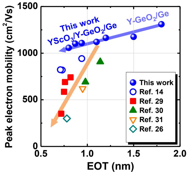
**Figure 3.17** Benchmarking of peak electron mobility in Ge n-MOSFETs as a function of EOT.<sup>14, 24, 27, 30-32</sup> Comparing to other conventional high- $k$ , YScO<sub>3</sub> shows moderate mobility degradation with reducing EOT.
