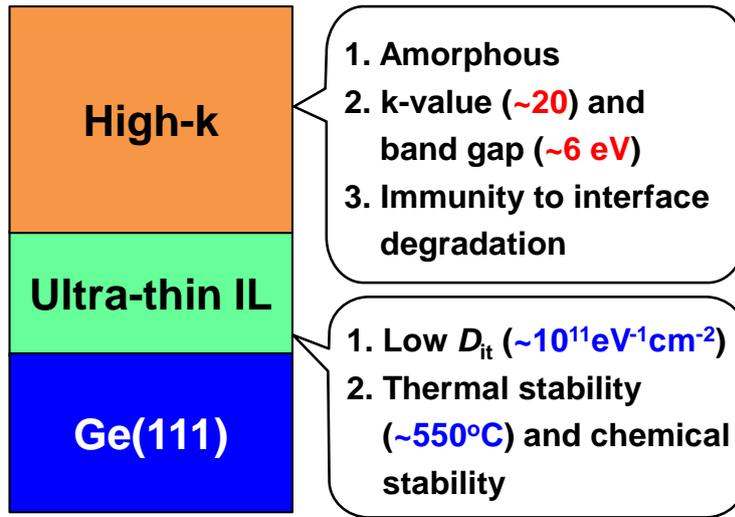
**Figure 3.1** Schematic of basic Ge gate stacks structure for EOT scaling into sub-nm region. The requirements on the ultra-thin IL and high-*k* are listed with regard to both IL and high-*k*. The issue for the IL has been addressed in the chapter 2.
