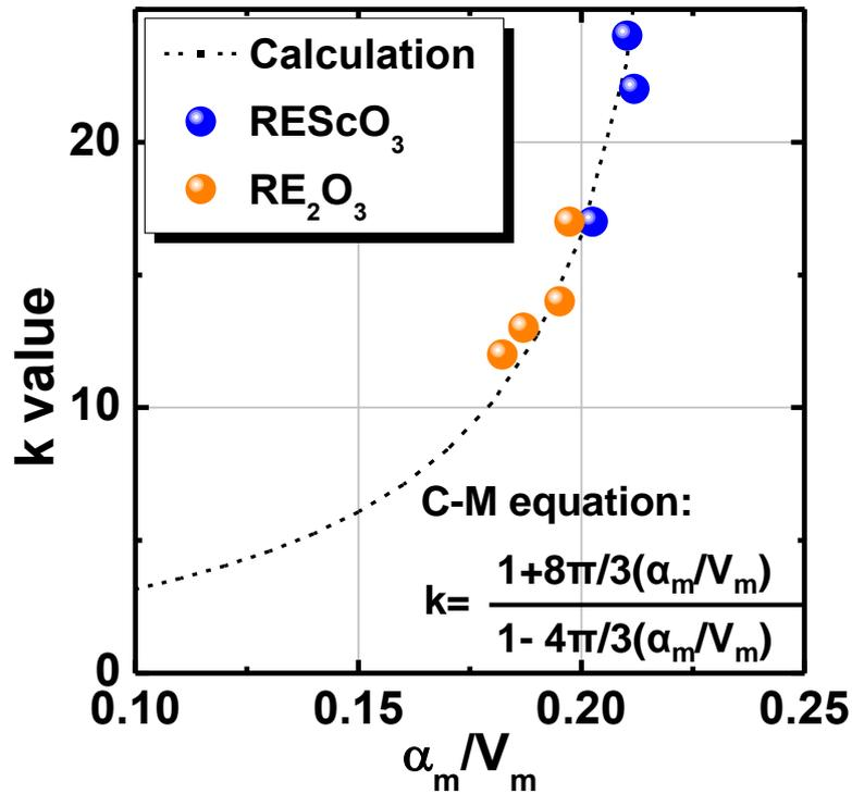
**Figure 3.11**  $k$ -value of  $\text{RE}_2\text{O}_3$ ,  $\text{Sc}_2\text{O}_3$  and  $\text{REScO}_3$  as a function of  $\alpha_m/V_m$  (ref. 18-21). The  $k$ -value predicted by C-M equation is also shown as a reference.
