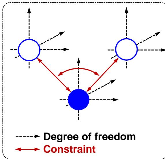
**Figure 2.28** Schematics of the degree of freedom and constrain of atoms in a network. The degree of freedom is related to the number of atoms, while the number of constraint is determined by the number of the bond.
