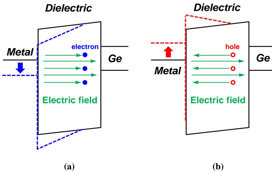
**Figure 4.1** Band diagram of Ge gate stacks with (a) electron or (b) hole trapping. Note that the black lines denote the ideal gate stack without trapping, while the blue and red dotted lines stands for the band distorted by electron and hole trapping, respectively. Such distortion of band is originated from the electric field from the trapped carriers, which is compensated by the shift of  $V_G$ .
