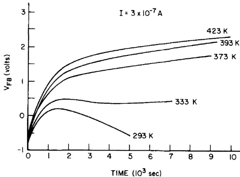
**Figure 4.2**  $V_{FB}$  shift of Al/SiO<sub>2</sub>/Si gate stack as a function of time under constant current stress of  $I=3 \times 10^{-7}$  A (gate diameter=0.032 inch).<sup>16</sup> For room temperature stress (293 K), the electron trapping is dominant initially and then the hole trapping becomes the major component.
