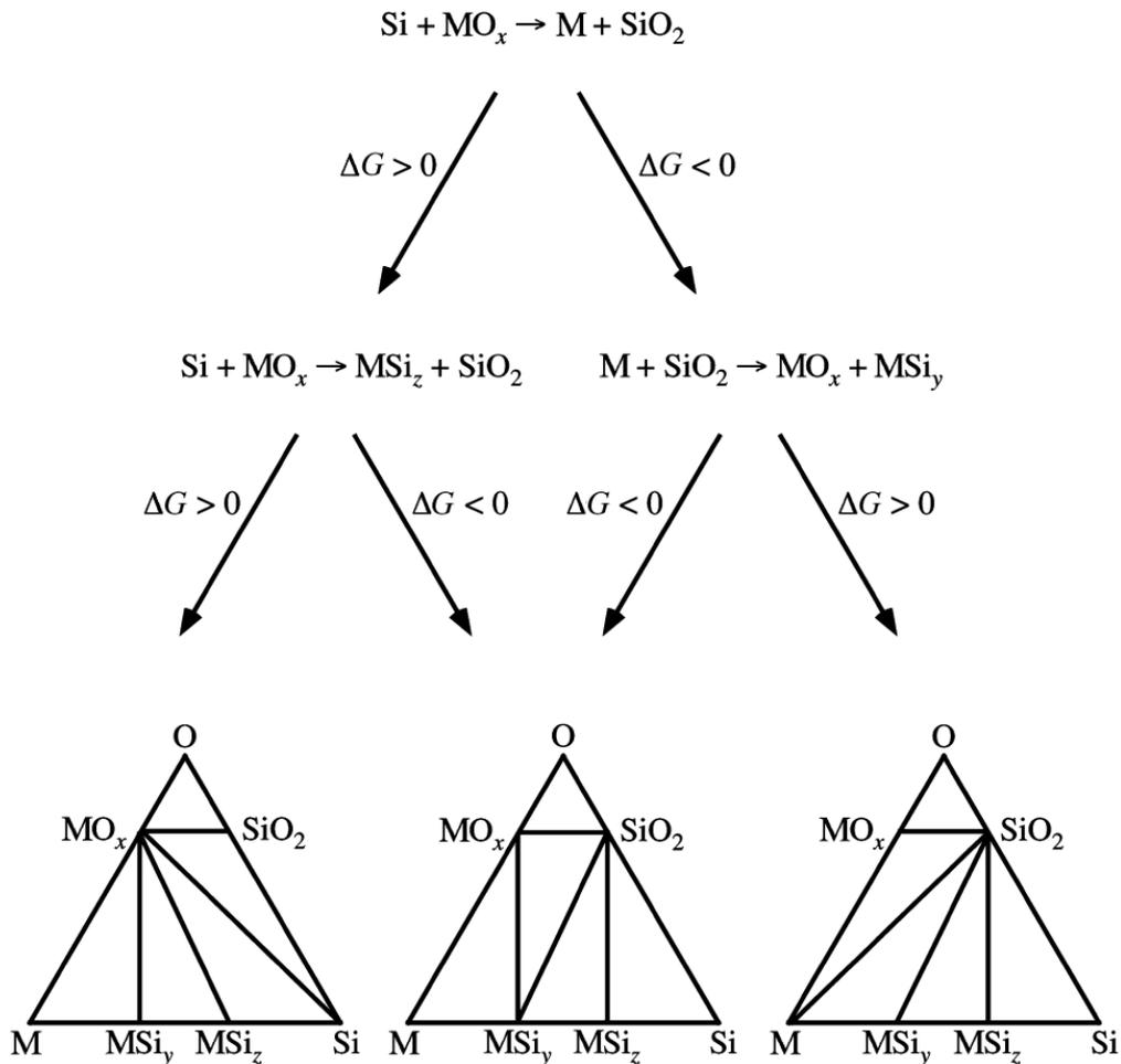
**Figure 3.2** Flowchart for the selection of thermally stable metal oxides on Si.<sup>8</sup> In the triangular diagram, a solid line is plotted between every two materials which are not reactive with each other.
