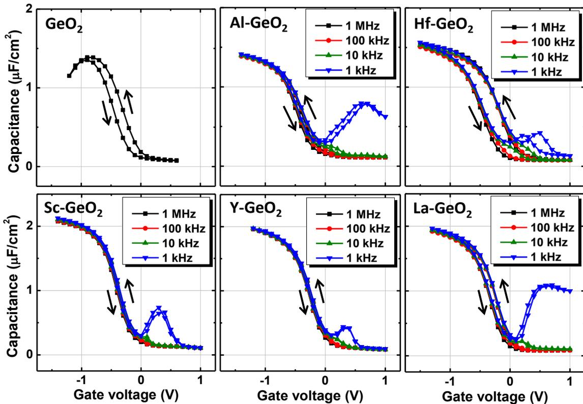
**Figure 2.24** Bidirectional *C-V* curves of Au/GeO<sub>2</sub>/Ge and Au/M-GeO<sub>2</sub>/Ge MOSCAPs measured at RT: (a) GeO<sub>2</sub>, (b) Al-GeO<sub>2</sub>, (c) Hf-GeO<sub>2</sub>, (d) Sc-GeO<sub>2</sub>, (e) Y-GeO<sub>2</sub>, (f) La-GeO<sub>2</sub>.<sup>12</sup> Note that the thicknesses of the dielectrics are about 3 nm in these gate stacks.
