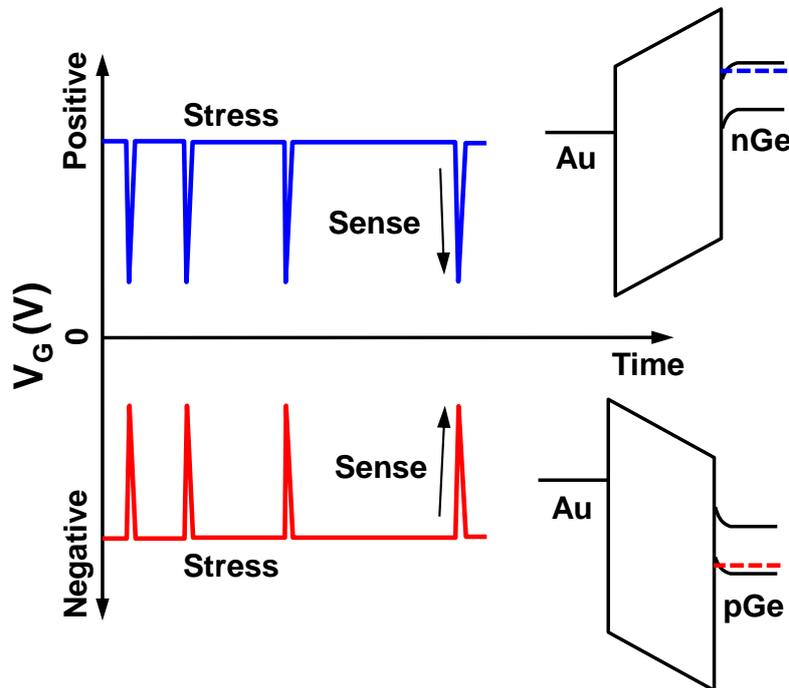
**Figure 4.5** Schematics of the experimental procedures for  $E_{\text{stress}}$  on Ge with both polarities.
