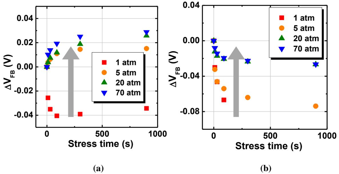
**Figure 4.7**  $V_{FB}$  shift in  $\text{GeO}_2/\text{Ge}$  stacks with various process  $P_{\text{O}_2}$  (1 to 70 atm) as a function of time under (a) positive and (b) negative  $E_{\text{stress}}$ . The large negative  $V_{FB}$  shifts are reduced in both polarities by increase  $P_{\text{O}_2}$ , which might be explained by less  $V_{\text{O}}$  formation during the gate stack process.
