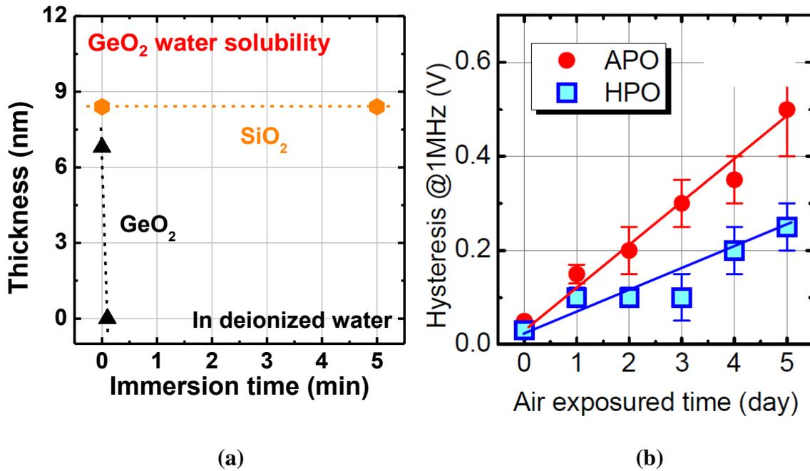
**Figure 1.7(a)** The thickness of  $\text{GeO}_2$  and  $\text{SiO}_2$  as a function of immersion time in DIW.  $\text{SiO}_2$  is not etched by water, while  $\text{GeO}_2$  is etched immediately. **(b)** Hysteresis of the  $C$ - $V$  curves of  $\text{GeO}_2/\text{Ge}$  gate stack as a function of time with exposure to air.<sup>41</sup> Regardless of the good initial properties, the hysteresis increase a lot with air exposure.
