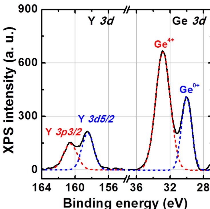
**Figure 2.5** XPS core level spectra of Y3d and Ge3d from a Y-GeO<sub>2</sub>/Ge stack. The spectra are deconvoluted as shown in the dotted curves.<sup>12</sup>
