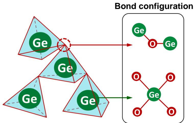
**Figure 2.15** Schematics of amorphous GeO<sub>2</sub> structure. The bond configurations of Ge and O atoms are also shown (2-dimensional represent).
