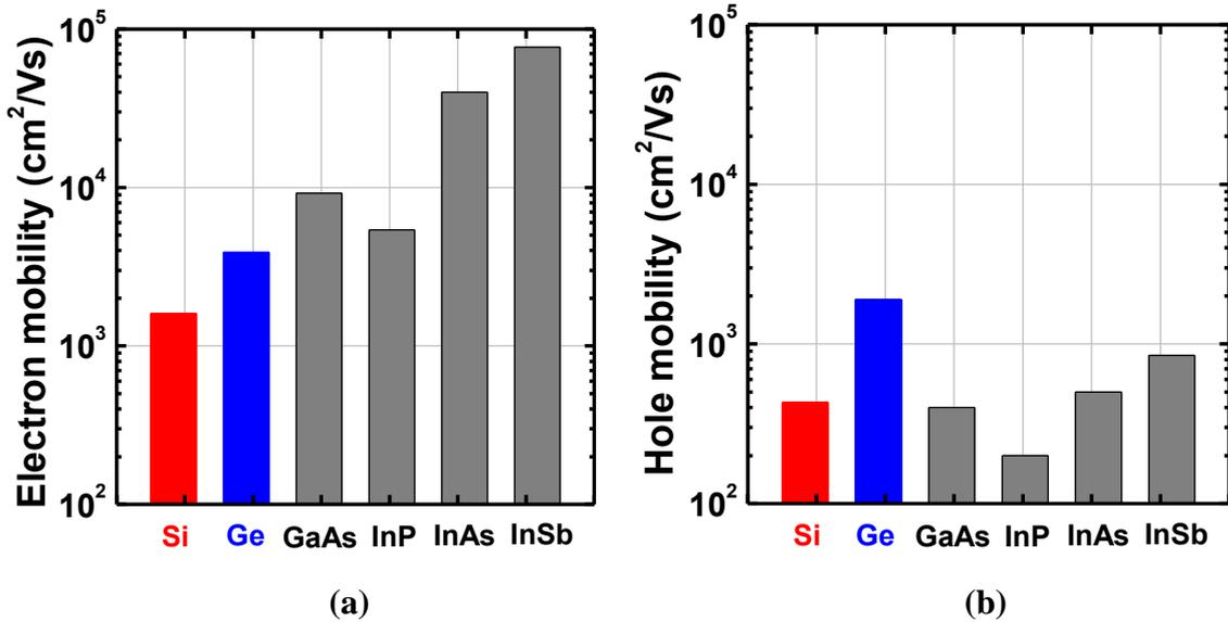
**Figure 1.4** Bulk mobilities of (a) electron and (b) hole for various semiconductors. The striking advantage of Ge over the other semiconductor materials is that its electron and hole mobilities are higher than Si in a balanced way.
