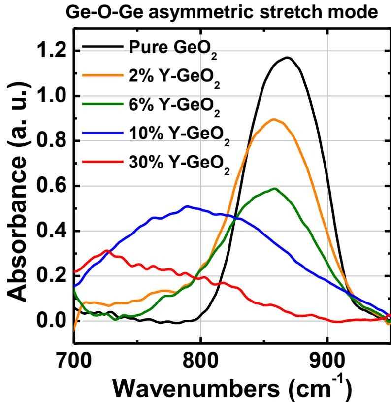
**Figure 2.18** FTIR absorbance spectra of pure GeO<sub>2</sub> and Y-GeO<sub>2</sub>.<sup>14</sup> The peak shift of asymmetric stretching mode in GeO<sub>2</sub> to lower energy is clearly observed with the increase of Y concentration. The thickness of the dielectrics are 40 nm
