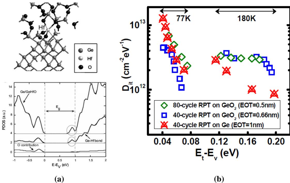
**Figure 1.8(a)** First principle calculations on the defect state formation when conventional high- $k$  dielectric ( $\text{HfO}_2$  in this case) was intermixed with  $\text{GeO}_2$  IL.<sup>46</sup> **(b)**  $D_{it}$  spectra of an aggressively scaled Ge stack with  $\text{ZrO}_2$  as high- $k$  (similar to  $\text{HfO}_2$ ).<sup>34</sup> Though very thin EOT is demonstrated, the  $D_{it}$  is in the order of  $10^{12} \text{ cm}^{-2} \text{ eV}^{-1}$  near the mid gap (almost 10
