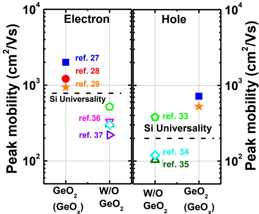
**Figure 1.5** Channel mobilities in Ge MOSFET reported in the literatures with high quality GeO<sub>2(x)</sub>/Ge interface<sup>27-29</sup> or with other dielectric passivation.<sup>33-37</sup> Both high electron and hole mobilities over that of Si universality<sup>25</sup> have been demonstrated by GeO<sub>2</sub>/Ge interface. While with other passivation methods, the mobilities are relatively poorer.
