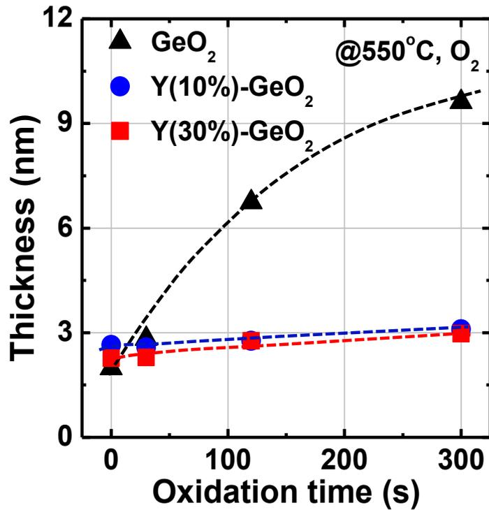
**Figure 2.9** Thickness of GeO<sub>2</sub> regrowth in (2 nm) Y-GeO<sub>2</sub>/Ge or GeO<sub>2</sub>/Ge stacks as a function of time under 550°C O<sub>2</sub> ambient annealing. Regardless of the same initial thickness of Y-GeO<sub>2</sub> and GeO<sub>2</sub>, the GeO<sub>2</sub>/Ge stack shows significant regrowth of GeO<sub>2</sub>, while Y-GeO<sub>2</sub> can block the further oxidation.
