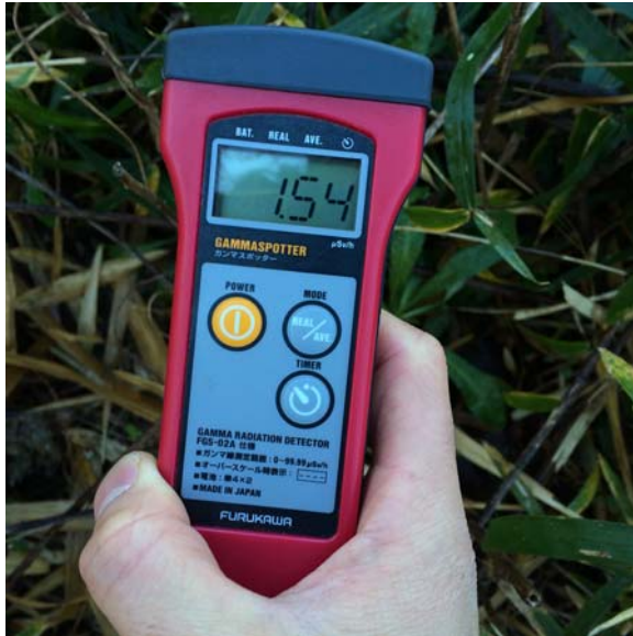
Figure 5.33: Measurement using personal dosimetry. Note, the measured vegetation were very close to the road. Higher dose has been observed in places close to the hot areas.
