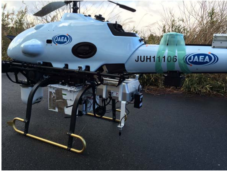
Figure 5.25: The newly developed wide area imager in the white enclosure mounted on the unmanned helicopter prior to take-off for the first flight measurement.
