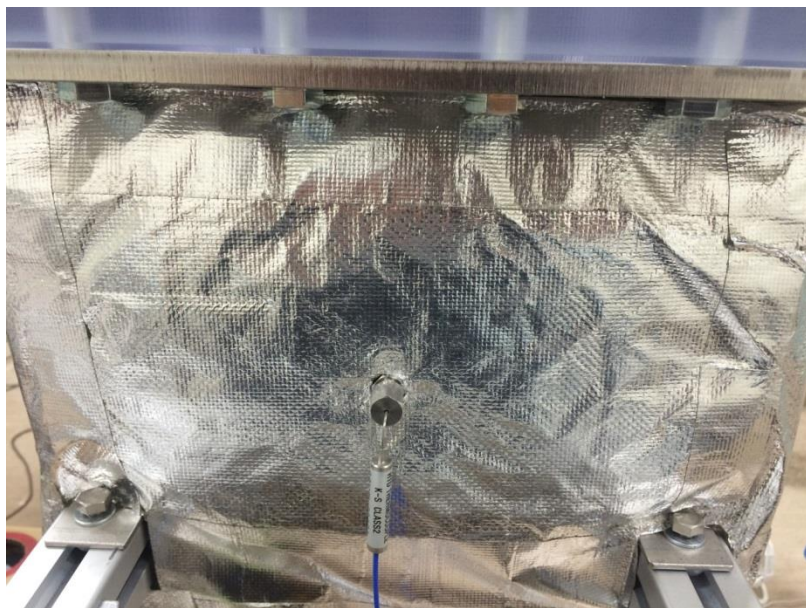
Figure 6-7: Thermocouple inserted in the upstream tank to monitor temperature of the water.
