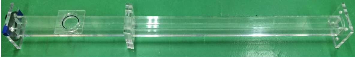
Figure 5-8: Longer portion (right) & shorter portion (left) of acrylic channel.
