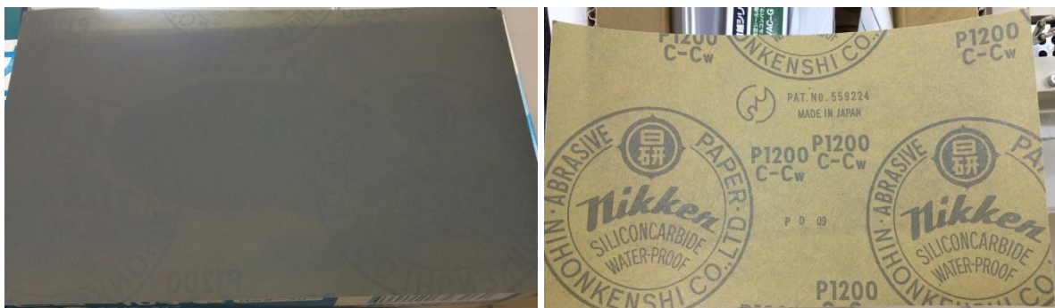
Figure 6-22: Front (left) and back (right) of P1200 sandpaper used to polish boiling surfaces.
