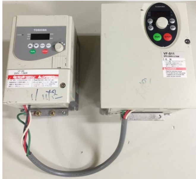
Figure 5-4: Individual controllers for each pump (not connected to pump when image taken).
