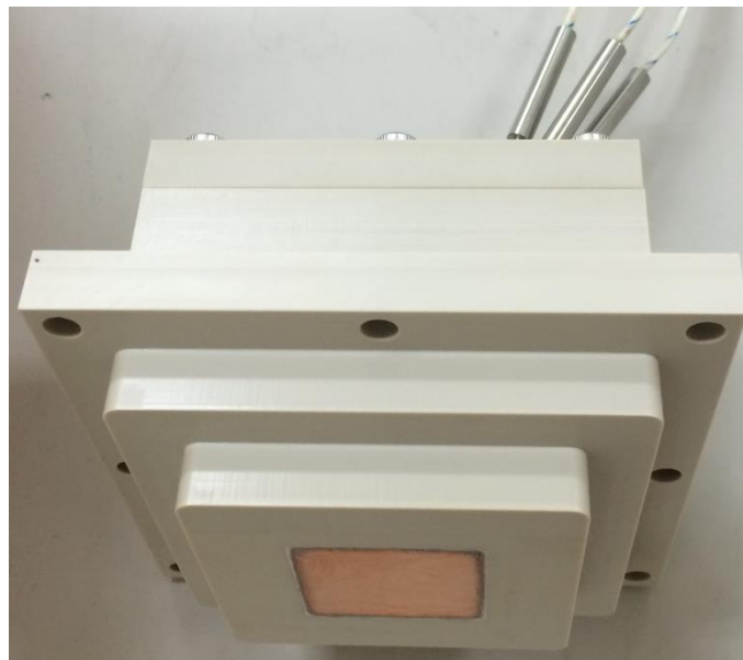
Figure 6-13: Image of PEEK enclosing the bare surface copper block.
