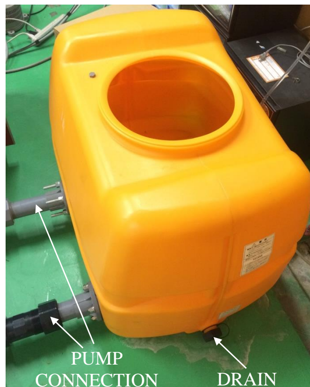
Figure 5-2: Image of water storage tank shown with the drain and pump connection.
