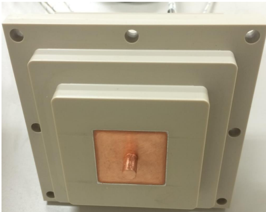
Figure 6-39: Image of PEEK enclosing the finned surface copper block.
