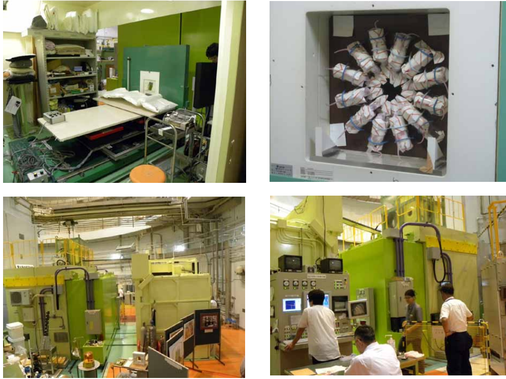
Figure 4.3: Nuclear reactor facility of Kyoto University Research Reactor Institute. Clockwise from top left: irradiation bed for patient treatment, irradiation setup for animal experiment on the neutron beam window, view of entrance door to the irradiation room, control panel and monitoring system during irradiation.
