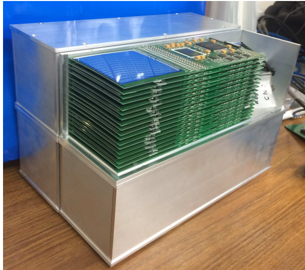
FIGURE 6.1: Imaging system composed of (2 \times 2) modules.
