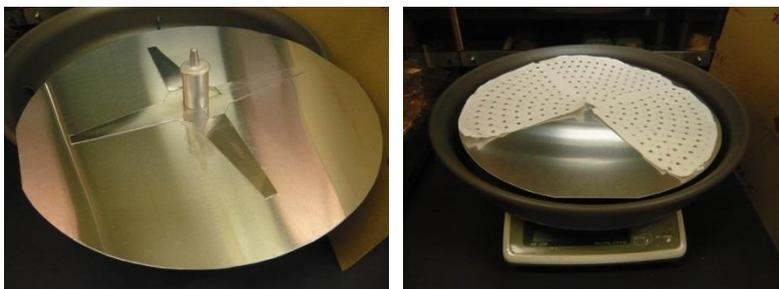
Figure 6 Custom aluminium weighing pan (bottom side) and filter on analysis balance with modified weighing chamber (filter already cut; top lid not attached).
