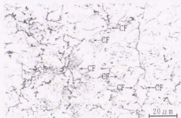
(C) Model 2 with 13 mass% carbonyl iron powder, 0.7 mass% ZnSt and 0.5 mass% liquid paraffin
