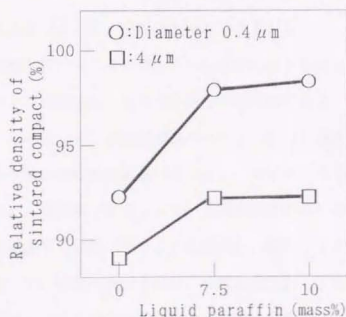
Fig.9-12 Effects of alumina particle diameter and liquid paraffin content to relative density of sintered cup-compact by compacting pressure of 196 MPa
