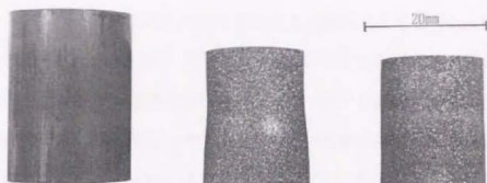
(A) Green compact (Non liquid paraffin) (B) Sintered compact (Non liquid paraffin) (C) Sintered compact (10 mass% liquid paraffin)
