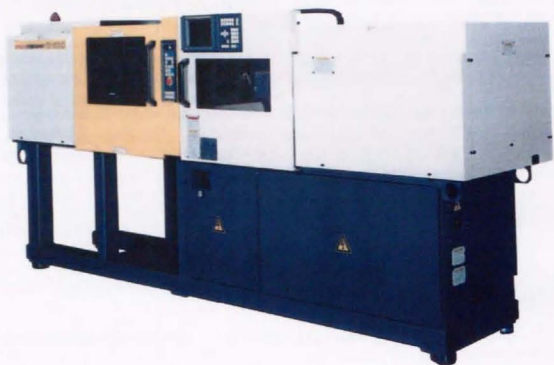
Fig.8 Outward appearance of the electric servo injection molding machine
