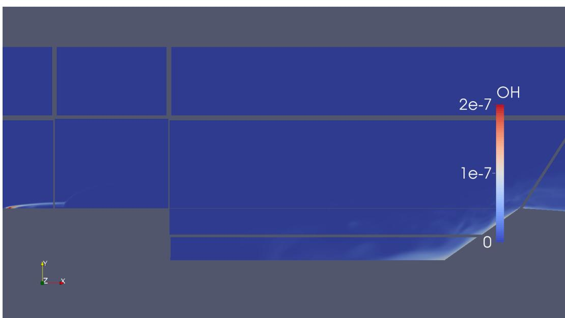
FIGURE 14: Hydroxyl radical distribution of Li-Williams combustion model results. The images show mass fraction of OH on xy plane passing the center of combustor.
