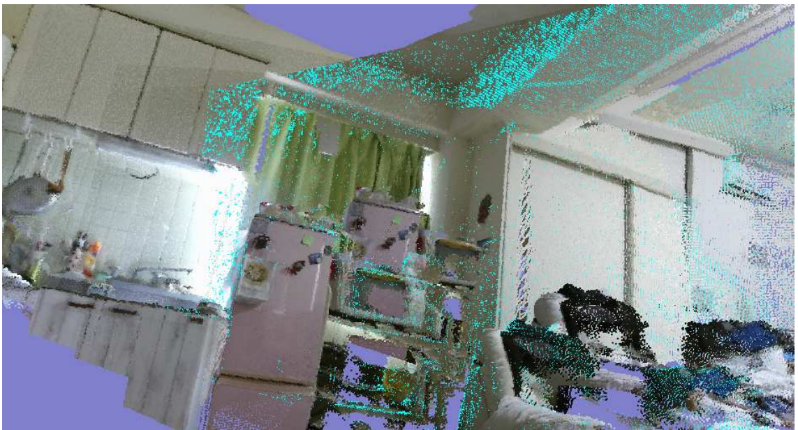
图 6.5: Looping back trajectory. Loop closure issue occurs.
