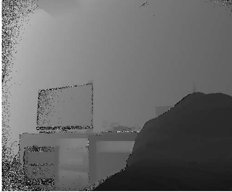
图 3.7: Raw input from Kinect 2 sensor
