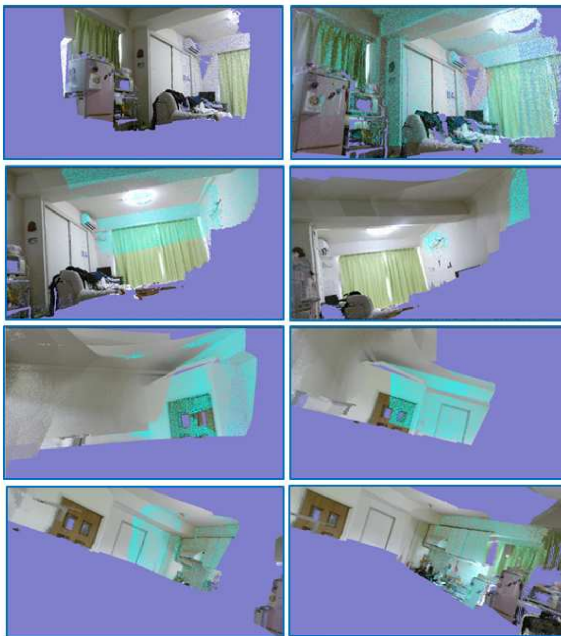
图 6.7: Step by step reconstruction of a room sized environment.
