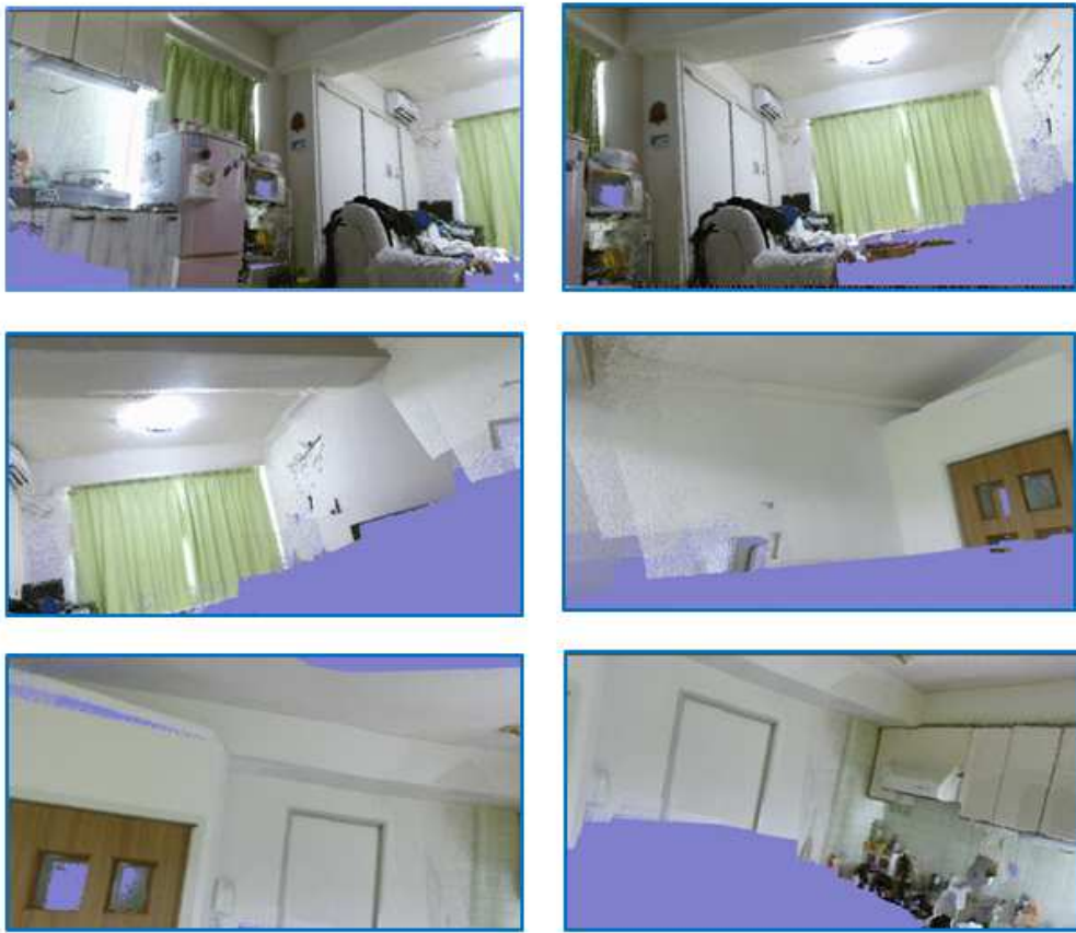
图 6.11: Step by step reconstruction of a room sized environment.
