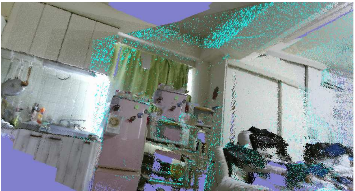
图 6.5: Looping back trajectory. Loop closure issue occurs.
