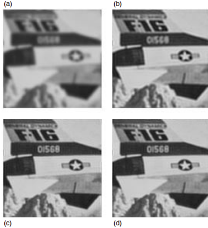
Figure 2.13: Blurred and restored images using RL. (a) blurred, (b) unaccelerated RL (250 iteration), (c) accelerated RL (250 iteration), (d) unaccelerated RL (10000 iteration)[4]
