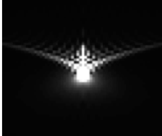
Figure 3.6: x - z profile of estimated PSF
