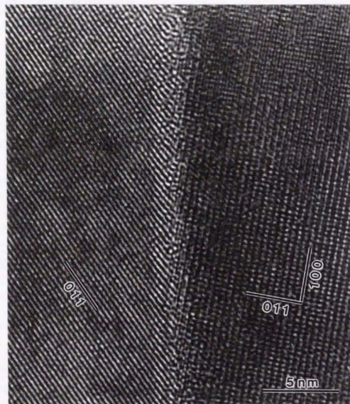
Fig. 3-4 High resolution electron micrograph of a grain boundary between the abnormal grains formed by the annealing at 1350°C × 6 h in 0.1%Nb- and 0.05%Ba-doped BaTiO 3 .
