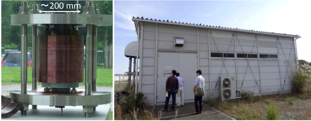
Figure 1.5: Left: A picture of a conventional pulsed magnet [72]. The inner coil is backed up with a maraging steel ring, and its outer diameter is typically \sim 200 mm. Right: a picture of a conventional capacitor bank of 500 kJ at SPring-8 BL19LXU.
