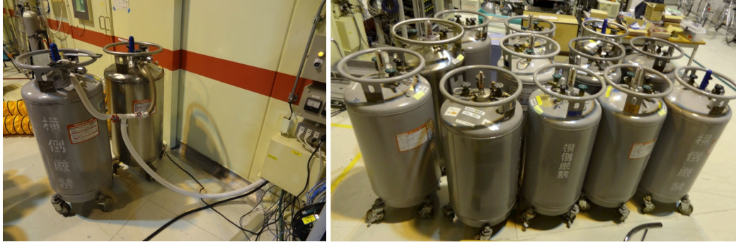
Figure 3.13: Vessels of liquid nitrogen placed at the outside of EH1. Left: a pair of vessels is used for a rapid switching. The hose goes through the duct. Right: 12 vessels are repeatedly filled by a supplier.
